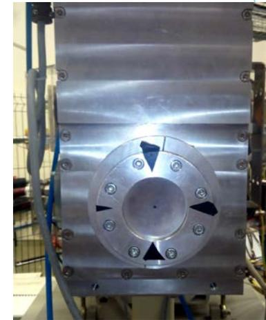
Protons scattered on the 50  $\mu\text{m}$  thick titanium foil of the beam-line exit window were used.
