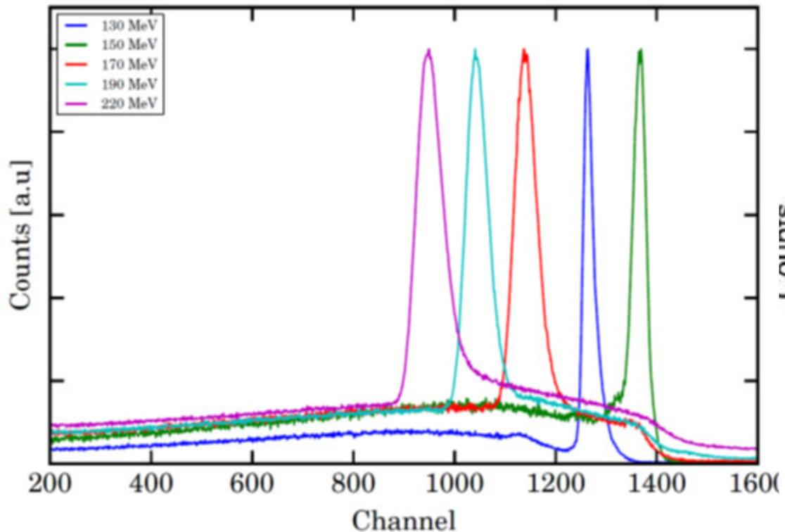
2"x2"x2" LaBr<sub>3</sub> - protons of energy above 145MeV are punch-through the detector. The spectrum for the 130 MeV protons is shown for comparison.
