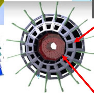
LaBr<sub>3</sub>/LaCl<sub>3</sub> + PMT
