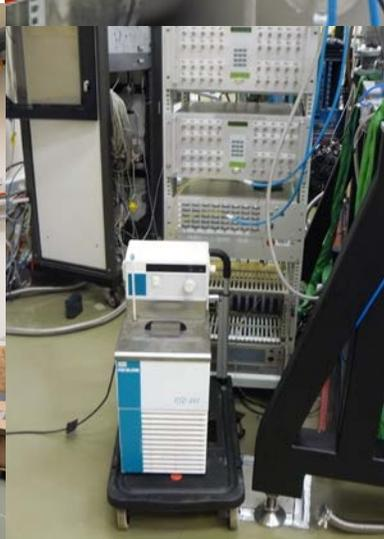
Only a 48V power supply is needed together with a chiller to keep under control the temperature of the FEE using a recirculating water circuit
