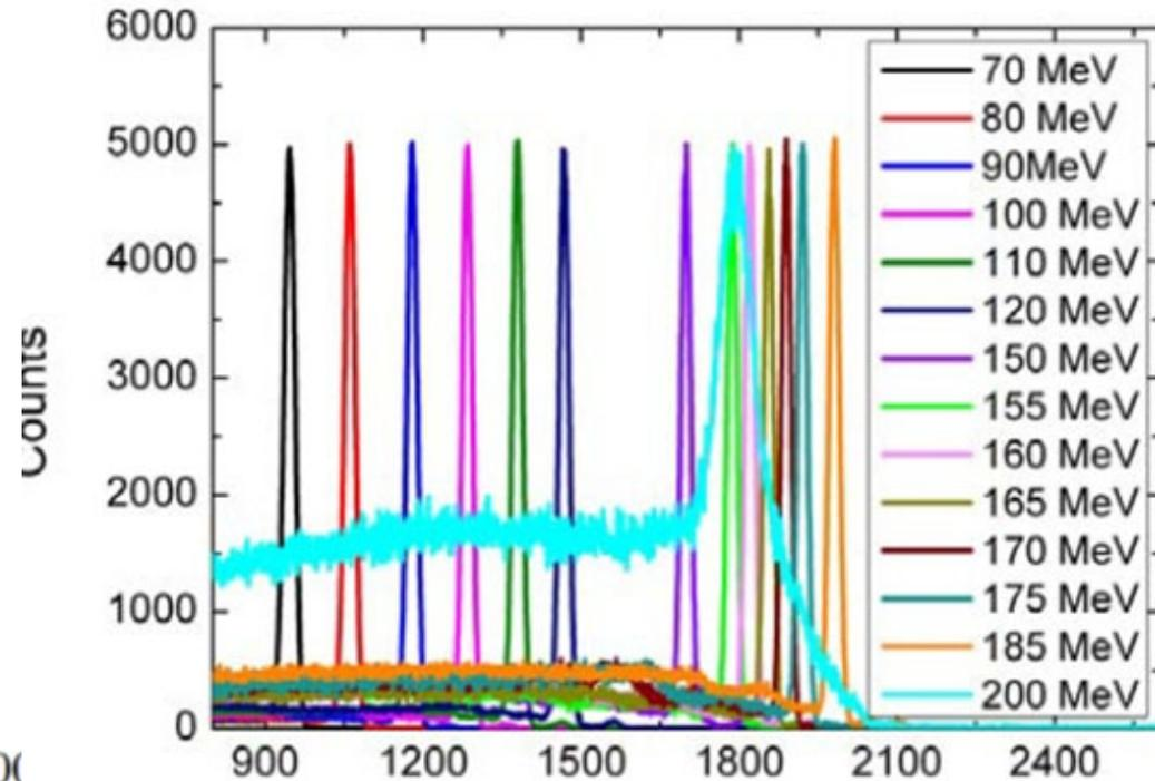
3"x3" LaBr<sub>3</sub> - protons of energy 70-185MeV are stopped inside the detector
