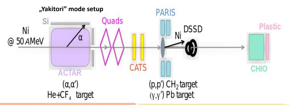
The first part of the setup will be dedicated to the measurement of ISGMR in the given Ni isotope and consists of the active target ACTAR.
