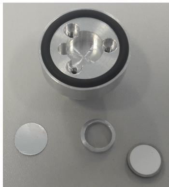
**Figure 3:** View of the original target holder with (from the left) cover plate, pressure ring and CaCO<sub>3</sub> target.
