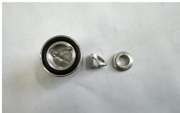
**Figure 2:** View of the new target holder with pressure and twisting rings.
