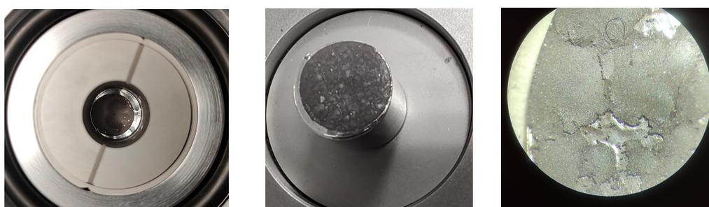
**Figure 4:** Dry Si deposit from toluene medium in the matrix ready for pressing (left), the deposit after compacting (middle) with clearly visible islands of grouped powder and magnification of the Si powder after press compacting (right). The small voids are already visible in the deposit before compacting (left).
