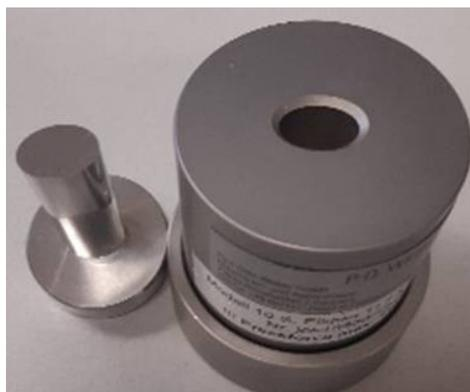
**Figure 4:** Die with shape allowing production of pellets with an elliptical shape.
