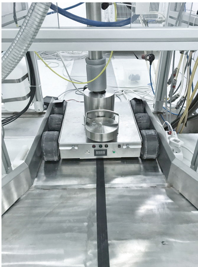
Figure 4: An irradiated target inside a lead container placed on the remotely controlled trolley.
