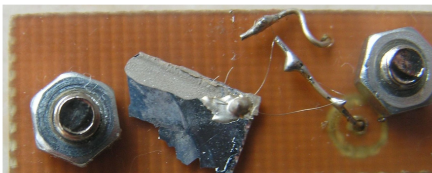
Figure 1: Thin epitaxial silicon detector with collimation cover removed with a 2 mm entrance hole. The 50 \mu\text{m} silver wire contacts were glued to both sides of the detector. The other ends of the wire contacts were soldered to a thick detector external wire connection.
