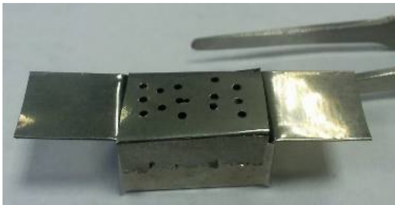
Figure 1: Crucible with perforated cover used for calcium carbonate conversion into oxide by resistant heating in vacuo.
