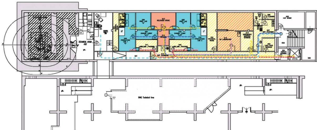
Figure 2: Layout of the RPRC. The proton/deuteron cyclotron and its control room is placed on the left part of the figure. Two independent production rooms are placed in the middle of the figure (the first one for the routine FDG production and the second one for other, also innovative, radiopharmaceuticals). The Quality Control room is placed in the right part of the figure (adapted from Refs. [2,4]).
