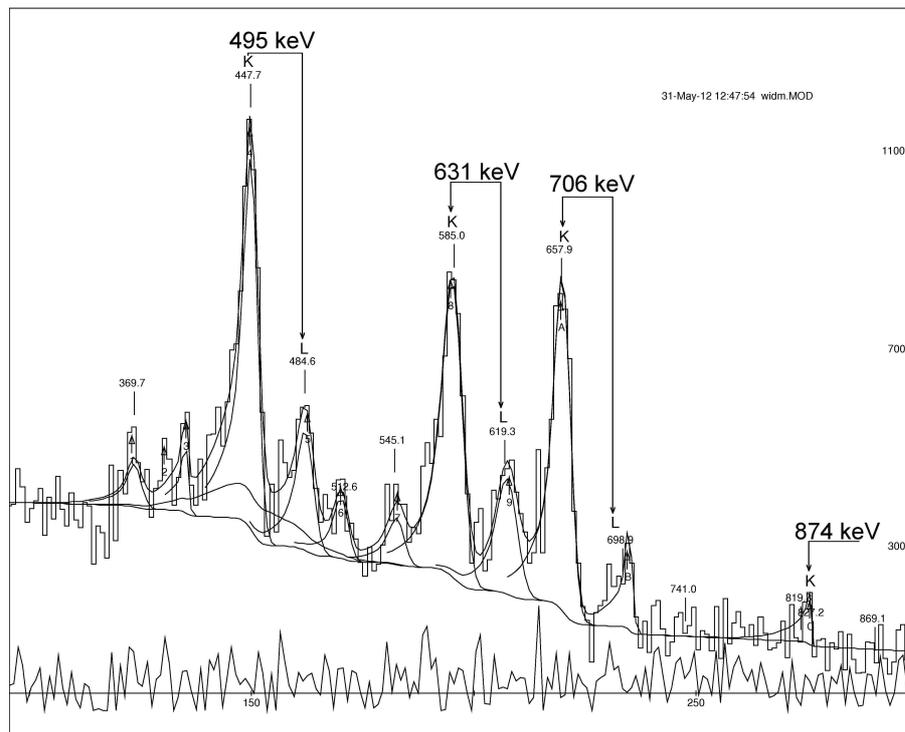
Figure 2: The summed “beam-off” electron spectrum in coincidence with the 294, 495 and 631 keV  $\gamma$ -ray transitions.
