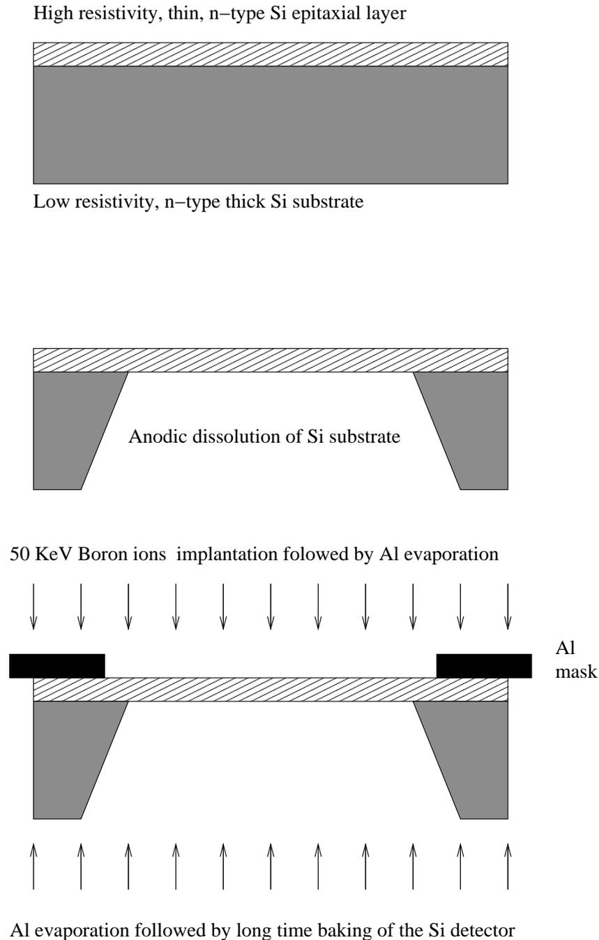
Figure 1: Technology of thin silicon detectors. We use  $n^+$ -n silicon structure (upper part of figure). The low-resistivity  $n^+$  substrate was removed by anodic dissolution (central part of figure) then 50 keV  $B^+$  ion implantation followed by Al metalisation was performed through Al mask on the n-type epitaxial 21  $\mu\text{m}$  silicon membrane. After Al metalisation of back side the wafer was baked during long time.
