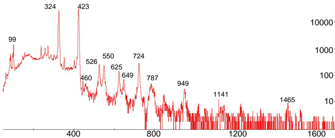
Figure 2: Gamma ray spectrum of  $^{107}\text{Ag}$  Coulomb excited by a  $^{32}\text{S}$  beam, summed over all HPGe and particle detectors. The  $\gamma$ -rays are in prompt coincidence with the scattered projectiles.
