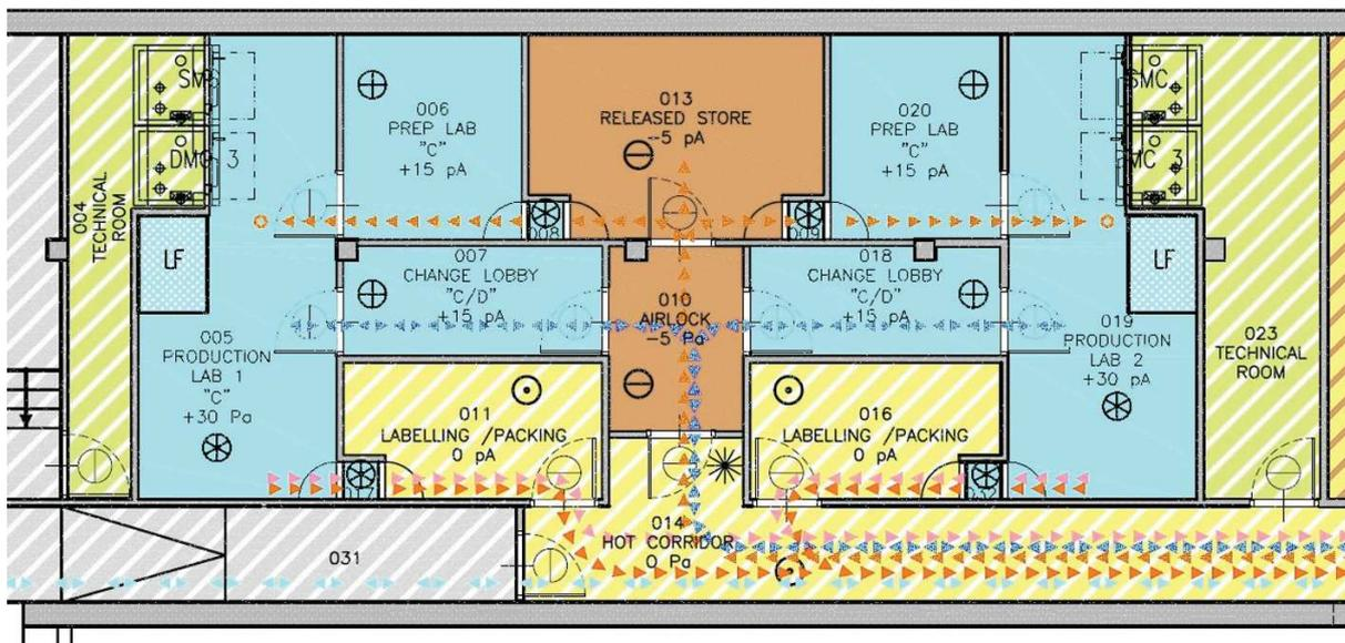
Figure 4: Enlarged view of the production rooms (adapted from Ref. [3]).
