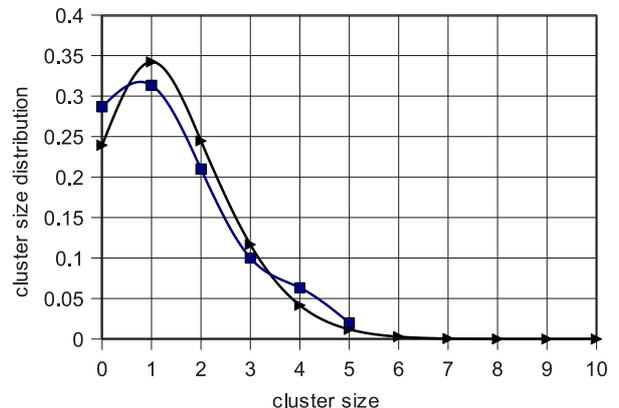
Figure 2: Frequency distribution of ionisation cluster size generated by alpha particles from At-211. Squares — experimental points, triangles — Poisson distribution for the mean cluster size.
