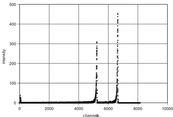
Figure 1: Measured spectra of alpha particles emitted by a sample with At-211
