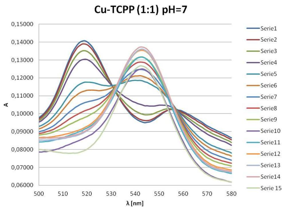
Figure 1: Kinetic spectra of Cu-Tetracarboxyphenyloporphyrin formation.
