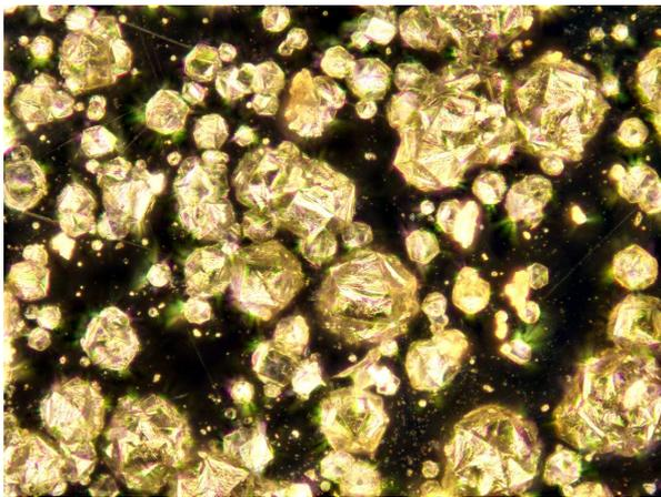
Figure 1: Diamond single crystals grown on a polished silicon surface.
