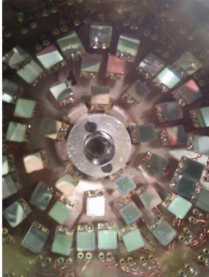
Figure 1: Backward hemisphere of the scattering chamber, with the degrader and PIN-diode detectors visible.
