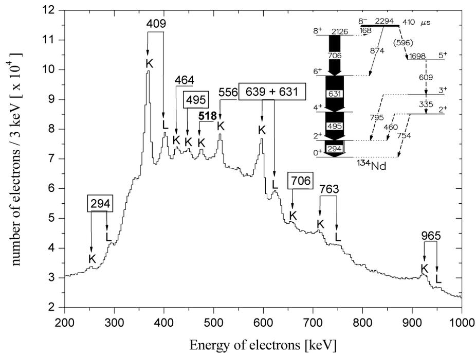
Figure 1: Total electron spectrum from the reaction:  $^{16}\text{O} + ^{122}\text{Te} \rightarrow ^{128}\text{Te}^*$ . The following lines may be recognised: decay of the isomeric state  $I^\pi = K^\pi = 8^-$  in  $^{134}\text{Nd}$  (text in rectangles), decay of  $^{134}\text{Pr}$  and decay of  $^{135}\text{Ce}$  (bold text).
