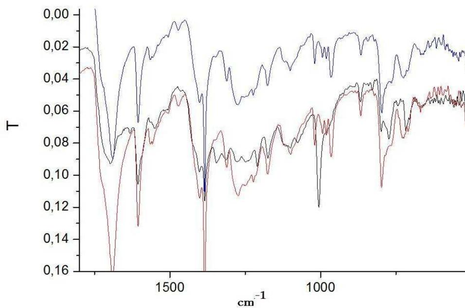
Figure 2: FT-IR spectra of tetracarboxyphenyloporphyrin (blue, red) and Ga-Tetracarboxyphenyloporphyrin complex.
