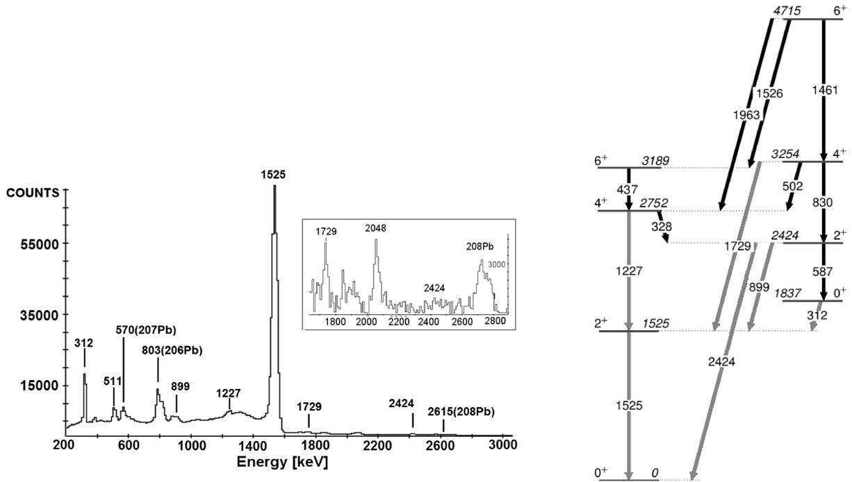
Figure 1: Left panel: a Doppler-corrected  $\gamma$ -ray spectrum observed in the  $^{42}\text{Ca} + ^{208}\text{Pb}$  Coulomb excitation experiment. Right panel: The scheme of excited states in  $^{42}\text{Ca}$ . Transitions observed in the current Coulomb excitation experiment are marked in grey.
