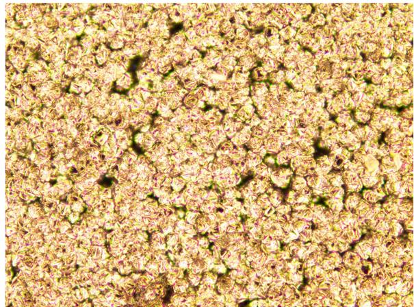
Figure 2: Diamond polycrystal layer grown on a lapped silicon surface.
