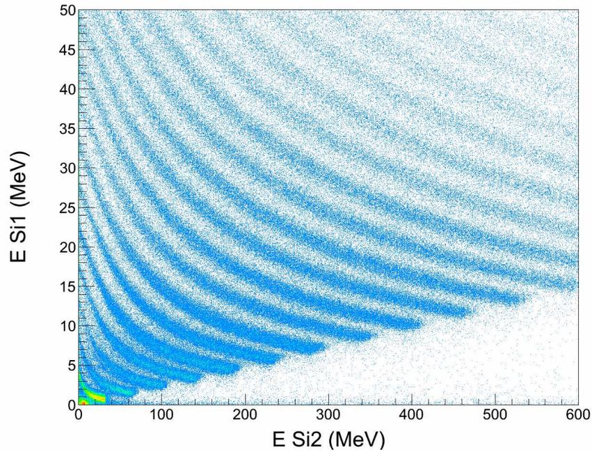
Figure 2:  $E-\Delta E$  scatter plot obtained using the  $E-\Delta E$  telescope consisting of  $21 \mu\text{m}$   $\Delta E$  detectors with an active area of  $20 * 20 \text{ mm}^2$  and a  $500 \mu\text{m}$   $E$  detector.
