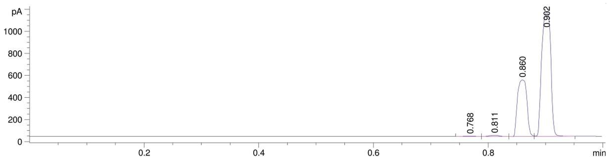
Figure 1: Gas-chromatographic separation of residual solvents. Signals, in order of appearance: methanol, ethanol, acetornitrile.
