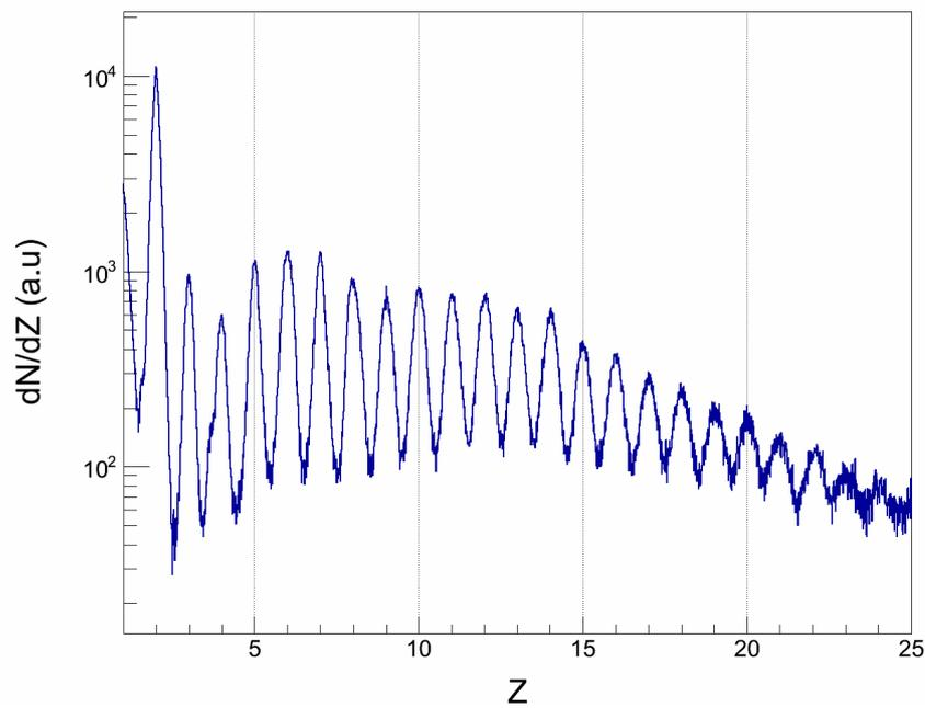
Figure 3: Charge distribution distribution of ions detected by the  $E - \Delta E$  telescope.
