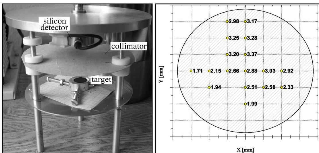
Figure 2: Right: set-up used for the determination of the energy loss of  $\alpha$  particles. Left: the thickness distribution of  $^{122}\text{Te}$  in the target.
