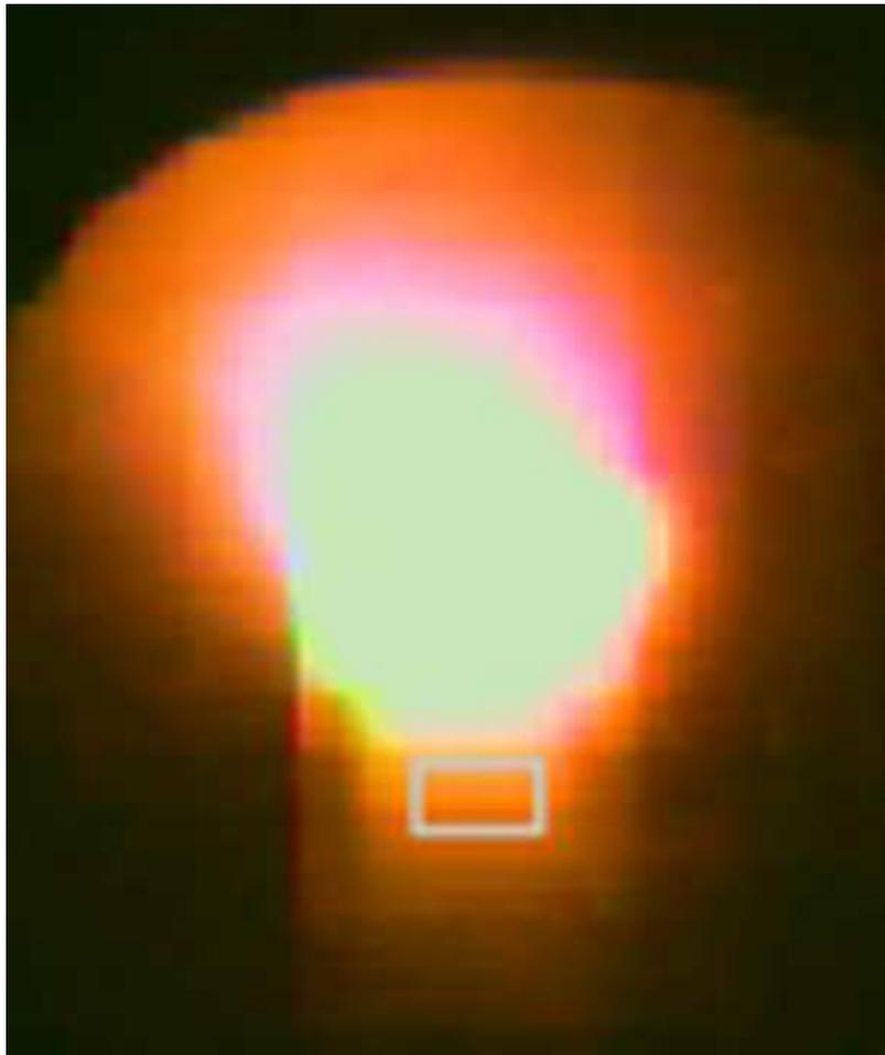
Figure 1: Picture registered by the WEB camera of the target heated to red colour by plasma during the Microwave Chemical Vapour Deposition process. The average value of light registered by pixels within the white rectangular frame is used for the temperature stabilisation of the target.
