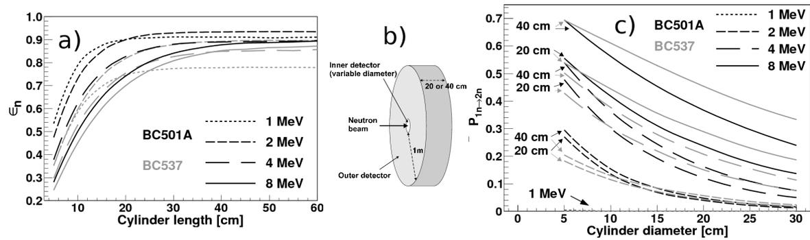
Figure 1: (a) Neutron detection efficiency as a function of detector length. (b) Setup used in the evaluation of the probability that one neutron generates a signal in more than one detector module. (c) Probability that a neutron shot onto the centre of the inner detector will generate signals in both detectors.
