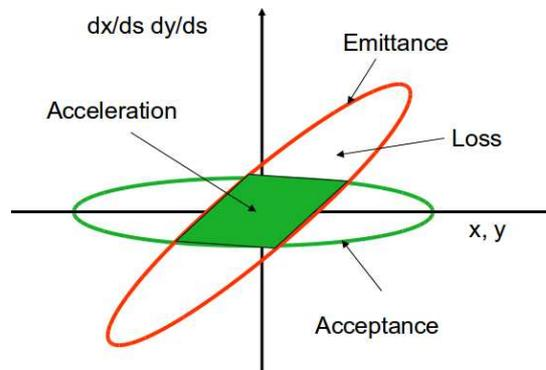
Figure 1: If the cyclotron acceptance in a given plane is like the green ellipse and the emittance of the beam is like the red ellipse, then only particles having the deviation-inclination coordinates within the overlapped green region will be accepted by the accelerating system.
