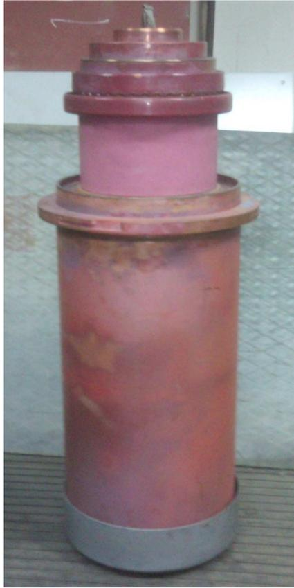
Figure 2: RF system power vacuum tube GK-11A from Dubna.
