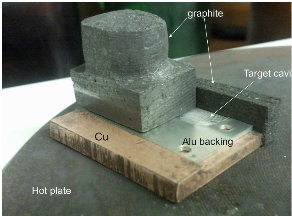
Figure 1: Production of the Bi target.
