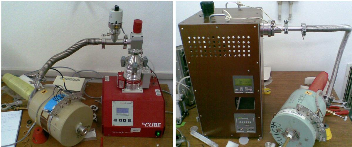
Figure 1: HPGe detector regeneration setups at HIL
