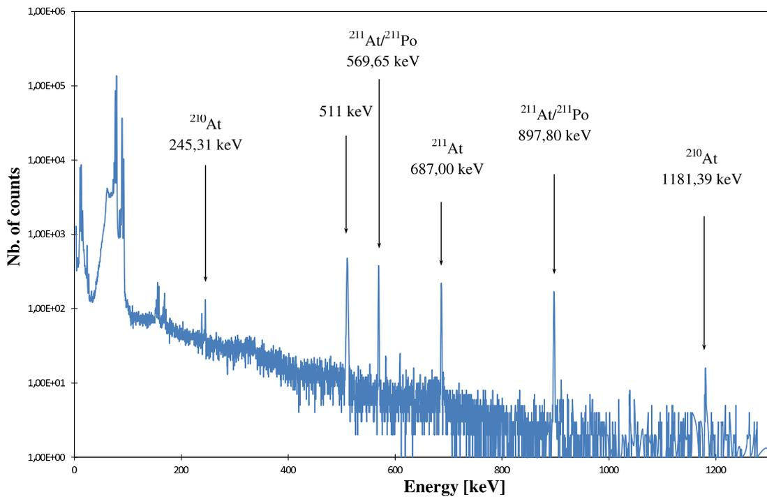
Figure 2: Gamma rays emitted from the  $^{209}\text{Bi}$  target shortly after irradiation with the 30 MeV  $^4\text{He}$  beam.
