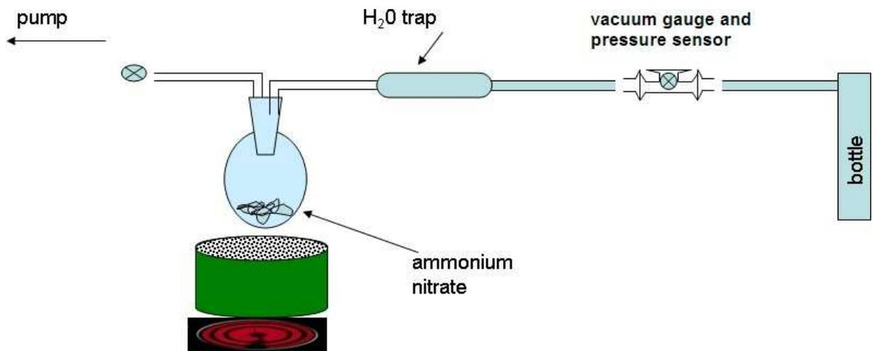
Figure 1: N-15 production set up.
