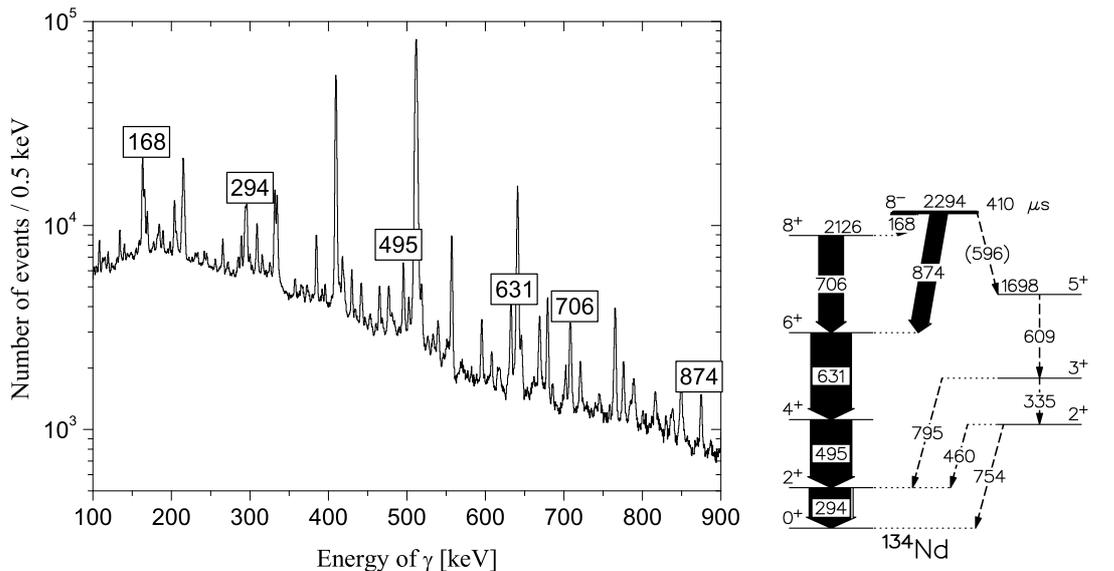
Figure 2: Gamma-ray lines observed with a  $^{122}\text{Te}$  target after 2 days’ exposure to a beam of  $^{16}\text{O}$  ions. The arrows indicate  $\gamma$ -ray transitions below the  $I^\pi = K^\pi = 8^-$  isomeric state in  $^{134}\text{Nd}$
