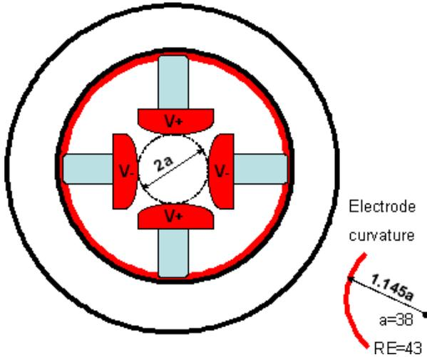
Figure 2: Schematic drawing of a single lens
