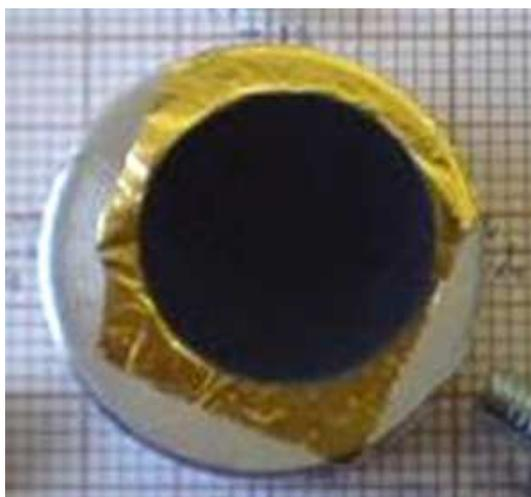
Figure 1: The  $^{122}\text{Te}$  target on gold foil backing mounted on the target holder.
