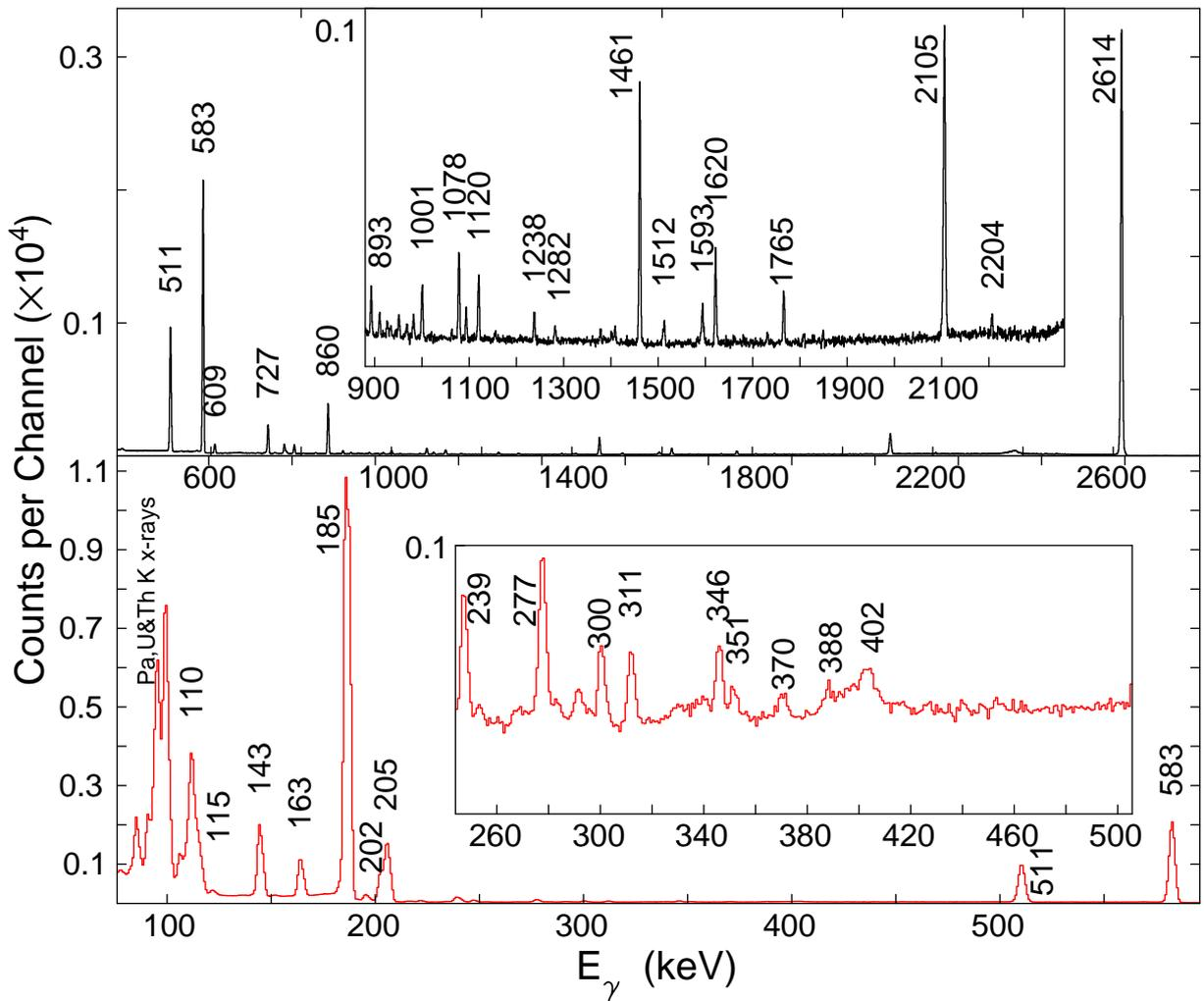
Figure 1: Example of  $\gamma\gamma$  efficiency corrected coincidence spectrum of 100 g Uranium sample, measured with 15 HPGe detectors.
