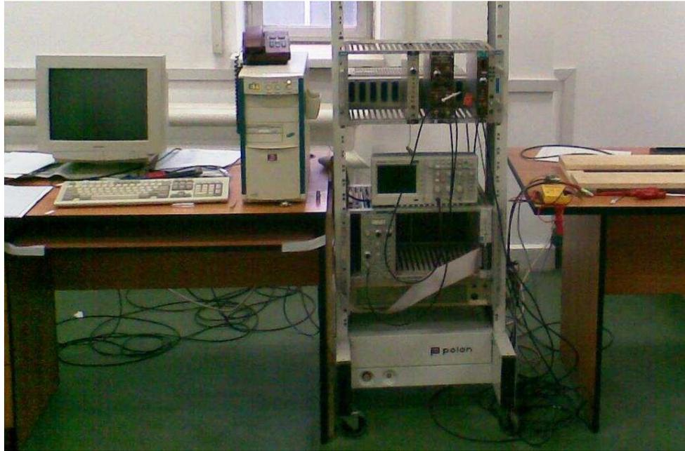
Figure 2: HPGe detector testing setup at HIL
