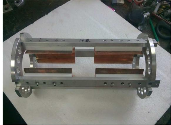
Figure 3: Photo of one of the two doublets installed in the cyclotron injection line.
