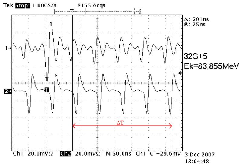
**Figure 1.** TOF method - a view from oscilloscope for  $^{32}\text{S}^{+5}$ :  $E = 83.9 \text{ MeV}$ . Time difference ( $\Delta T = 291 \text{ ns}$ ) used for energy determination is marked.
