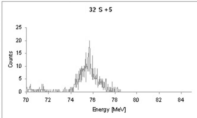
**Figure 2.** A sample spectrum from the beam scattering set-up ( $^{32}\text{S}^{+5}$  beam). To calculate the beam energy, the energy of scattered ions measured by the detector should be divided by a factor resulting from the scattering kinematics. In this case the factor is equal to 0.91, therefore  $E = 75.6 \text{ MeV} / 0.91 = 83.1 \text{ MeV}$ .
