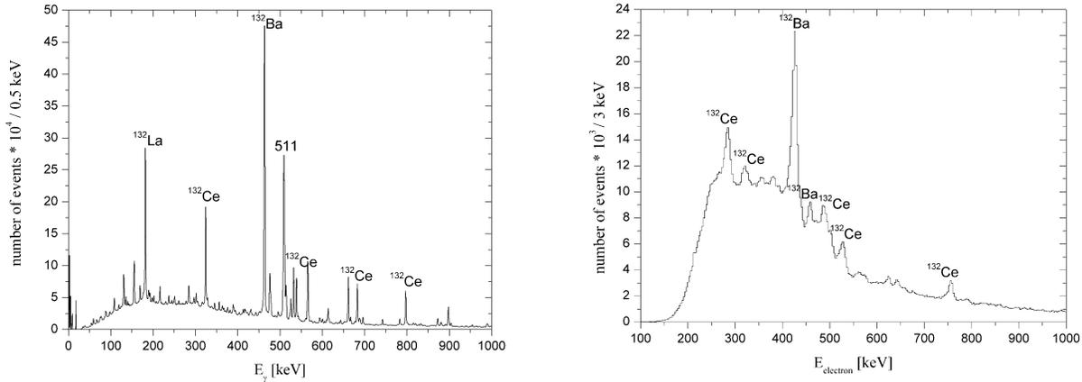
**Figure 3.** Left: The total gamma ray spectrum in coincidence with electrons from reaction  $^{120}\text{Sn}(^{16}\text{O},4n)^{132}\text{Ce}$ . Peaks from  $^{132}\text{Ce}$  and its daughter nuclei  $^{132}\text{La}$  and  $^{132}\text{Ba}$  are clearly visible. Right: The total electron spectrum in coincidence with gammas from the induced reaction. Internal conversion electron peaks from  $^{132}\text{Ce}$  and  $^{132}\text{Ba}$  are clearly visible.
