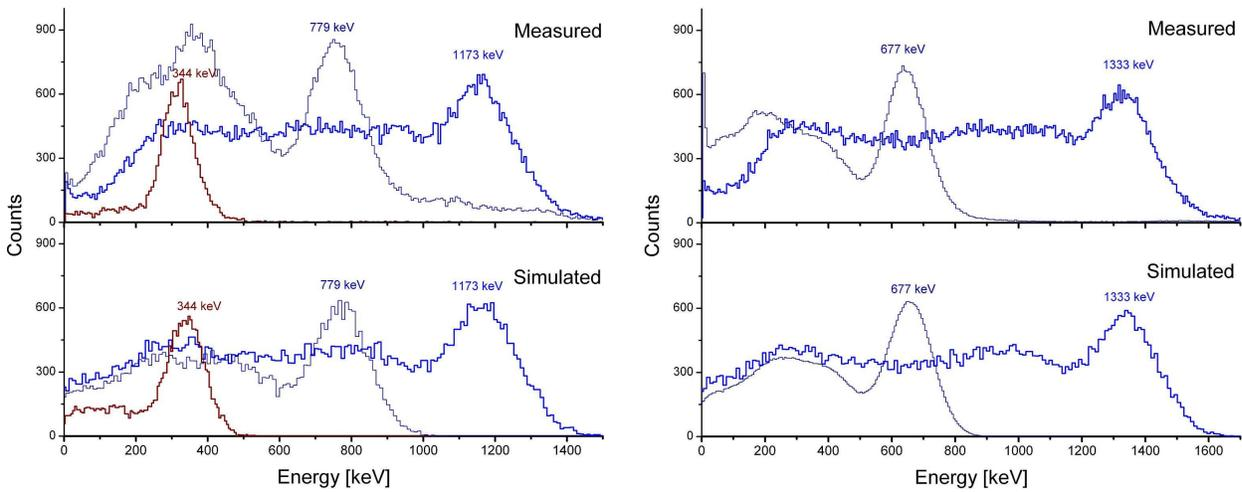
**Figure 1.** Measured and simulated (GEANT4)  $\text{BaF}_2$  energy spectra.
