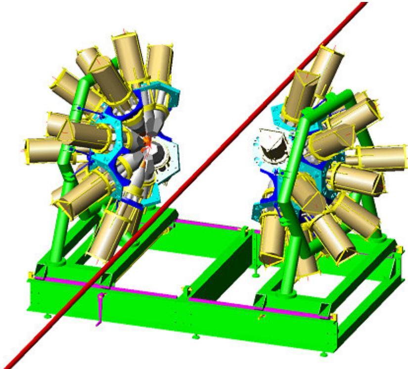
**Figure 1.** Final layout of the EAGLE array: configuration with 30 HPGe detectors.
