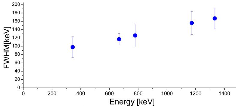
**Figure 2.** Energy resolution of one of the tested  $\text{BaF}_2$  crystals, shown as a function of  $\gamma$ -ray energy.
