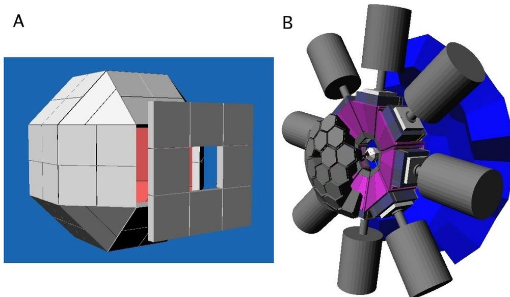
**Figure 1.** GEANT4 models of detectors: DIAMANT charged particle detector (a) and the AGATA Demonstrator combined with EXOGAM, Neutron Wall and DIAMANT (b).
