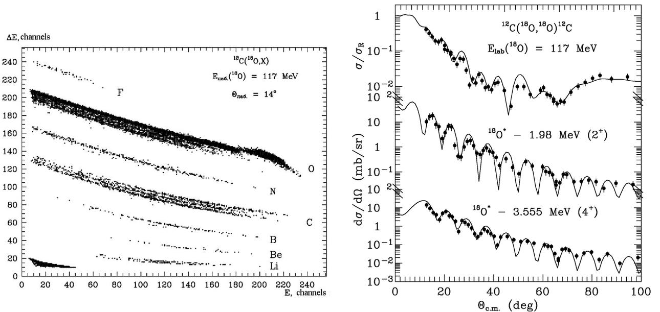
**Figure 1.** Left panel: Typical  $\Delta E(E)$ -spectrum of the  $^{12}\text{C}(^{18}\text{O}, X)$  reaction products at  $E_{\text{lab}}(^{18}\text{O}) = 117$  MeV. Right panel: Angular distributions of the  $^{12}\text{C} + ^{18}\text{O}$  elastic and inelastic scattering at  $E_{\text{lab}}(^{18}\text{O}) = 117$  MeV. The curves represent the OM- and CRC-calculations.
