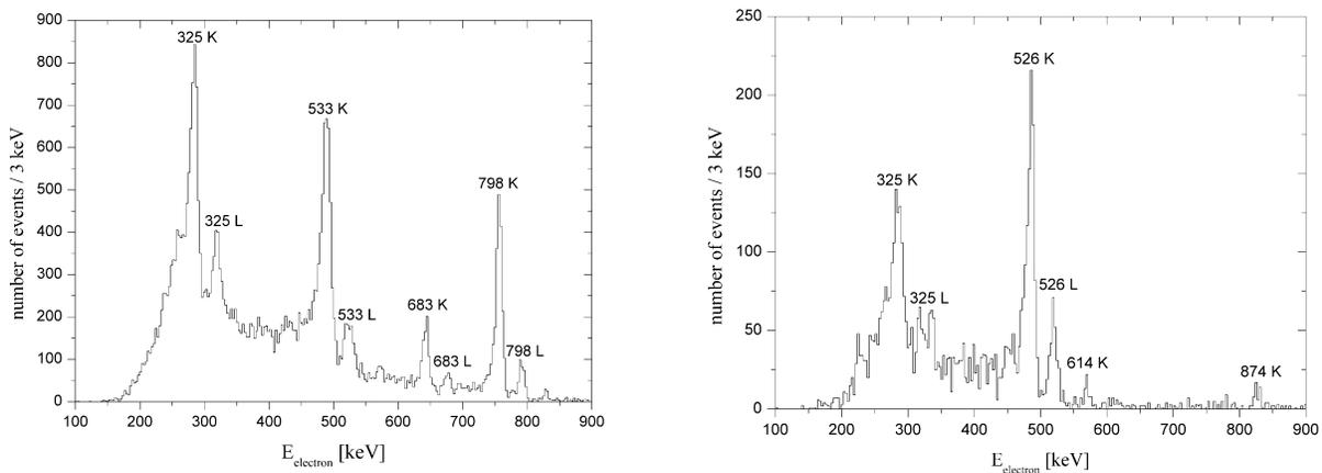
**Figure 4.** The electron spectra showing the K and L electron peaks descent from decay transitions of the K isomer in  $^{132}\text{Ce}$ . Left: The sum of spectra gated by 325, 533 and 683 keV gamma lines. Right: The sum of spectra gated by 614 and 874 keV gamma lines.
