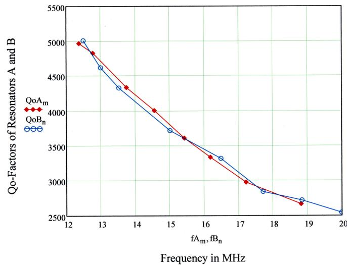
Figure 1. The Q factors of "A" and "B" resonators
