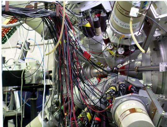
**Figure 2.** A photo of the experimental set-up. The internal conversion electron spectrometer (in the middle) is coupled to the OSIRIS-II array.
