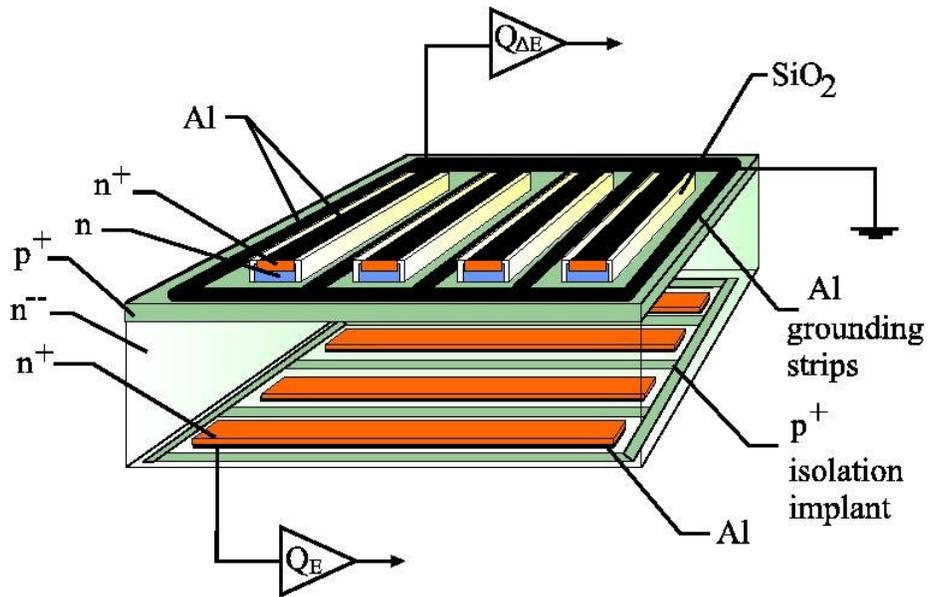
**Figure 3.** Design of the double-sided strip monolithic silicon E -  $\Delta E$  telescope produced by Quasi-Selective Epitaxy.
