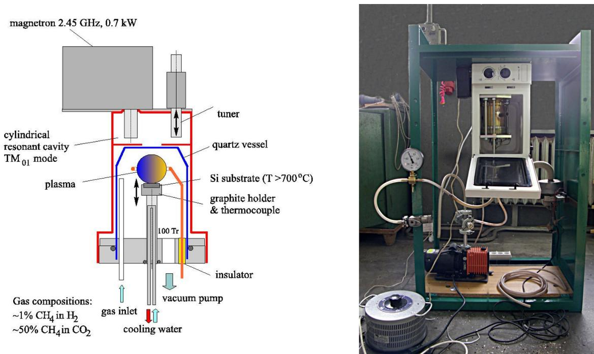
**Figure 1.** Design of the reactor for Microwave Chemical Vapour Deposition and photo of the device.
