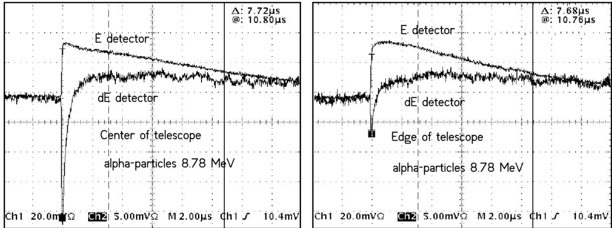
**Figure 2.** Oscilloscope pictures of the charge preamplifier outputs for a monolithic E -  $\Delta E$  telescope with a 20  $\mu\text{m}$  thick E- $\Delta E$  detector irradiated by  $\alpha$  particles of 8.78 MeV energy. For  $\Delta E$  detectors a negative cross-talk signal is observed. Left:  $\alpha$  particles hit the centre of the telescope. Right:  $\alpha$  particles hit the edge of the  $\Delta E$  detector.
