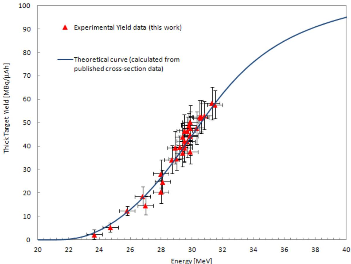
**Figure 1:** Experimental thick target yield [2] for the production of  $^{211}\text{At}$  by the  $(\alpha,2n)$  reaction on a Bi target. The theoretical curve was calculated using the cross-section data of Ref. [3].
