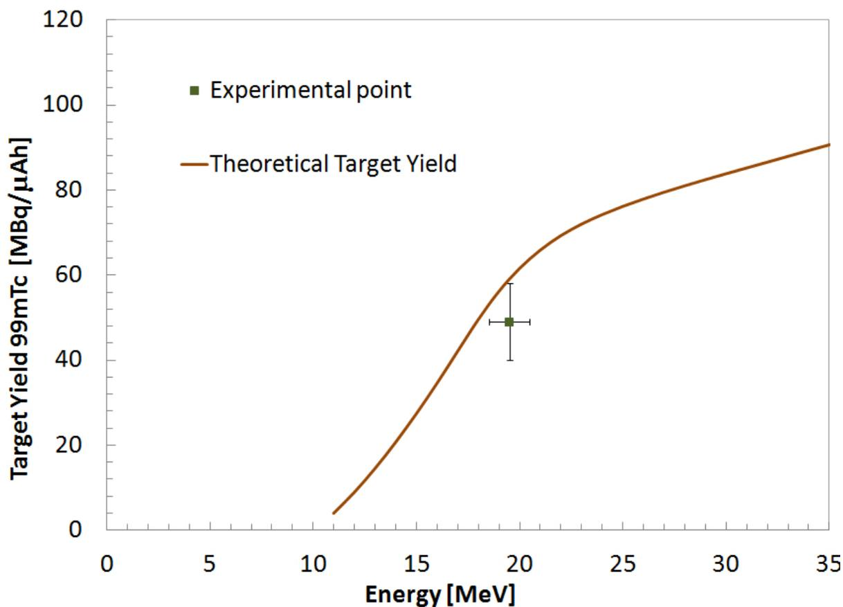
**Figure 4:** Comparison of the experimental and theoretical Target Yield for the production of  $^{99m}\text{Tc}$  from a  $^{\text{nat}}\text{Mo}$  target with a thickness of 500  $\mu\text{m}$  at a bombarding energy of 19.8–11.0 MeV.
