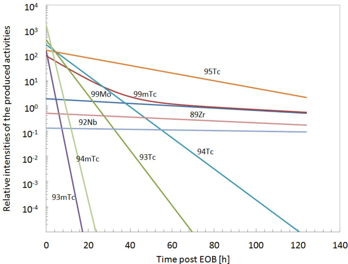
**Figure 3:** Activity balance of technetium radioisotopes as a function of time after a 0.22 h irradiation of a thick target at 19.84–10.99 MeV
