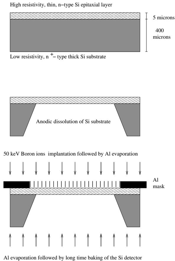
**Figure 1:** Technique of low-temperature for 5  $\mu\text{m}$  thick silicon strip detector production.
