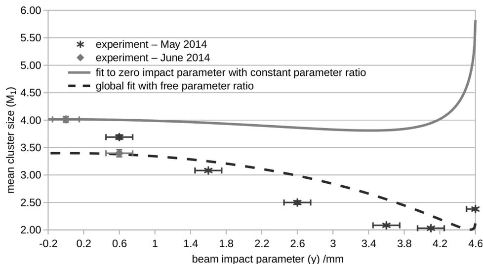
**Figure 1:** Data obtained in two experiments with the carbon ion beam at HIL. The curves represent two fits of the simple geometric model of the wall effect. The constant parameter ratio was obtained in the Monte Carlo simulation.
