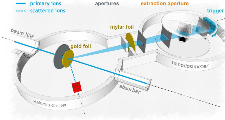
**Figure 1:** Schematic setup of the PTB nanodosimeter for measurements at an ion accelerator.
