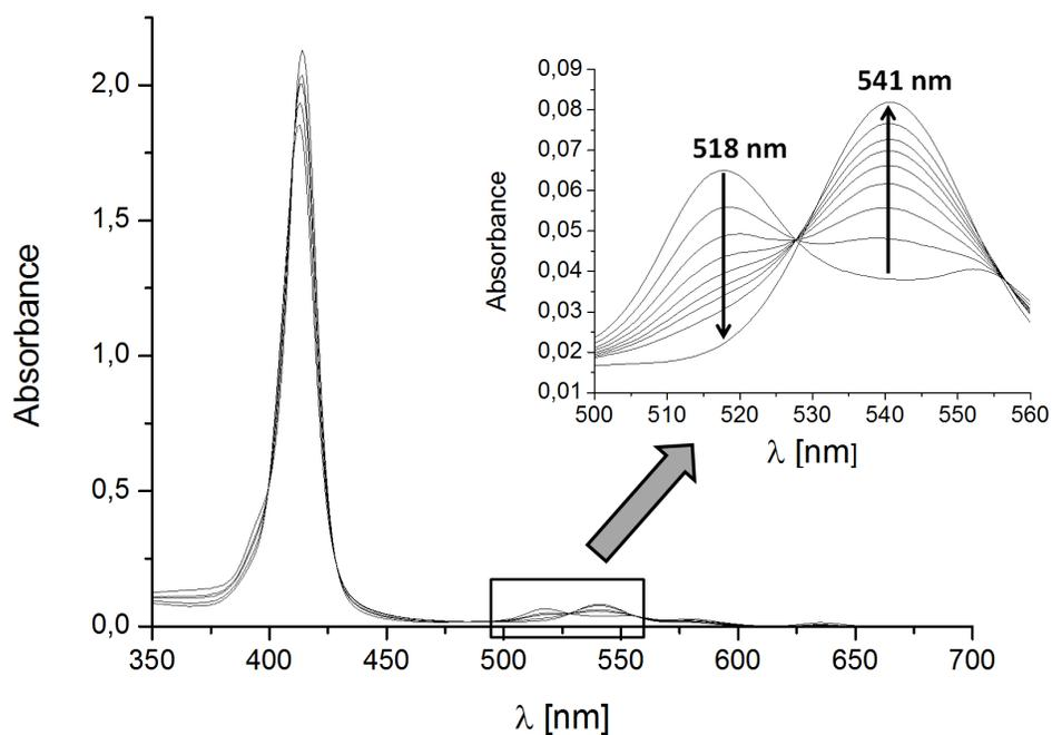
**Figure 1:** The formation of a CuTCPP complex with characteristic changes in the UV-VIS spectrum.
