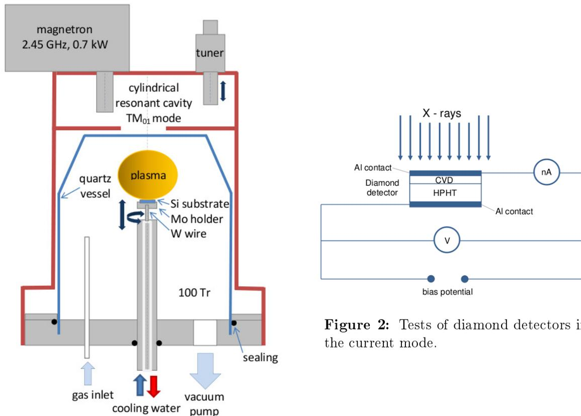
**Figure 1:** MWCVD reactor.
