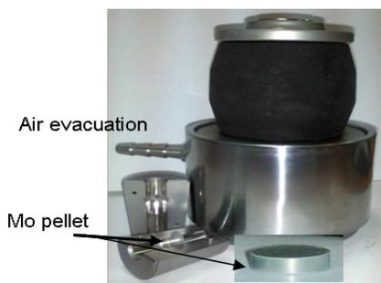
**Figure 1:** The pellet die with air evacuation option.
