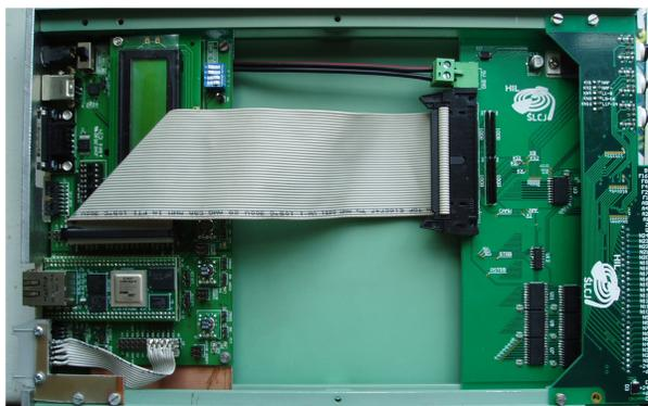
**Figure 2:** The new CAMAC Crate Controller.
