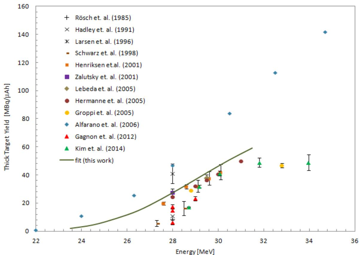
**Figure 2:** Comparison of previously published thick target yields for  $^{211}\text{At}$  production by the  $(\alpha,2n)$  reaction with the fit to the present experimental points, as presented in Fig 1.
