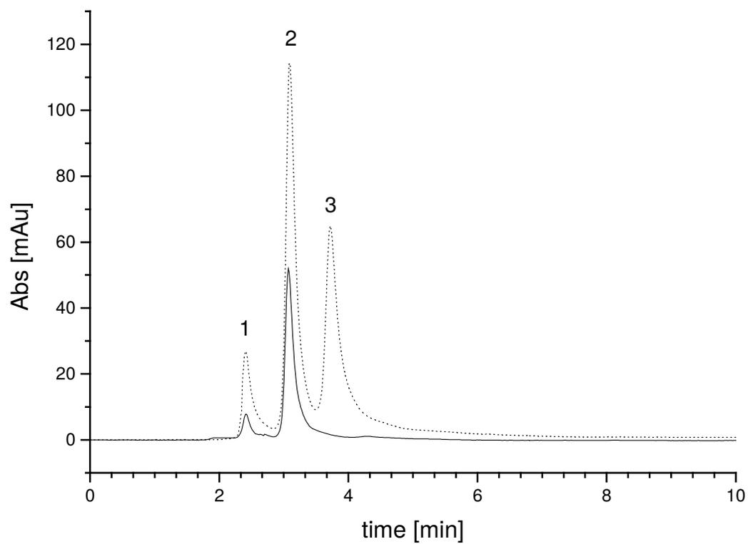
**Figure 1:** UV-Chromatogram of reference standards (dotted line) and  $^{11}\text{C}$ -metnionine sample (solid). 1-L-homocysteine (tr=2.51 min), 2-methionine (tr=3.05 min.), 3-L-homocysteine thiolactone hydrochloride (tr=3.72 min.)
