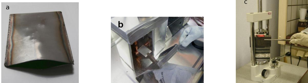
**Figure 3:** To flatten the Mo droplet at temperature, a droplet prepared by powder melting was packed into a stainless steel envelope (a) sintered tightly under an argon atmosphere (b). The packet was heated to 1100 °C and when hot, pressed under the hydraulic press (c).
