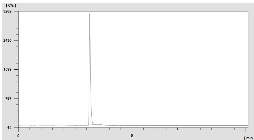
**Figure 2:** Radiochromatogram of  $^{11}\text{C}$ -methionine (tr=3.07 min)
