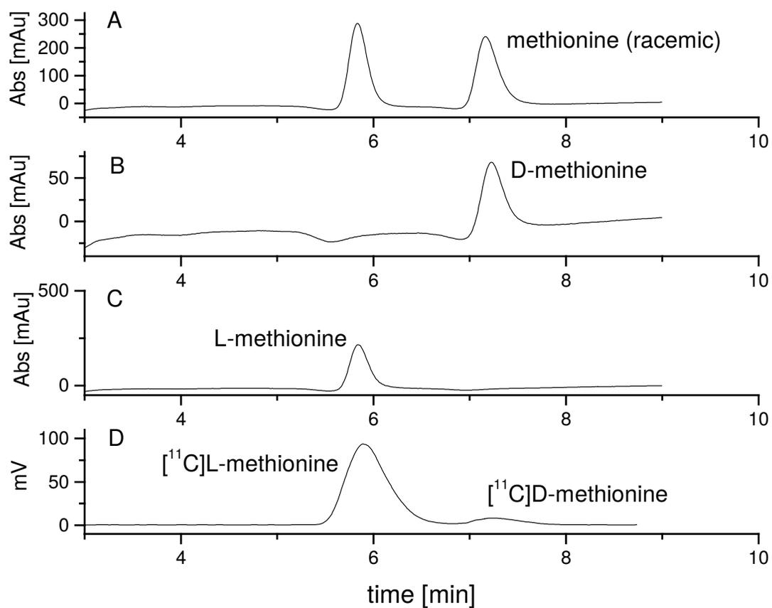
**Figure 3:** Standard and sample chromatograms for enantiomeric purity evaluation. (A) UV spectra of racemic methionine CRS, (B) UV spectra of D-methionine CRS, (C) UV spectra of L-methionine CRS, (D) Radiochromatogram of  $^{11}\text{C}$ -methionine sample.
