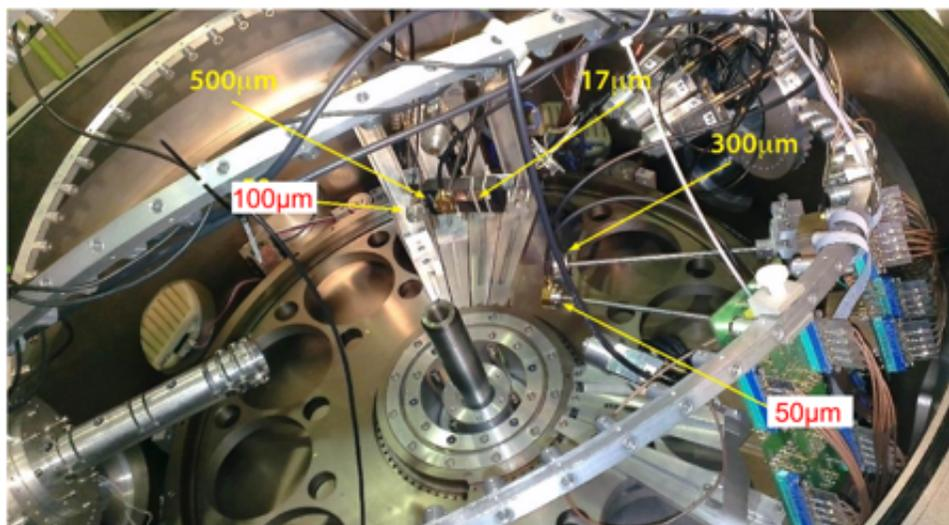
**Figure 1:** The experimental set-up used for the scCVD detector test at the Heavy Ion Laboratory, University of Warsaw. Detectors used for the coincidence measurement are labelled in white boxes.
