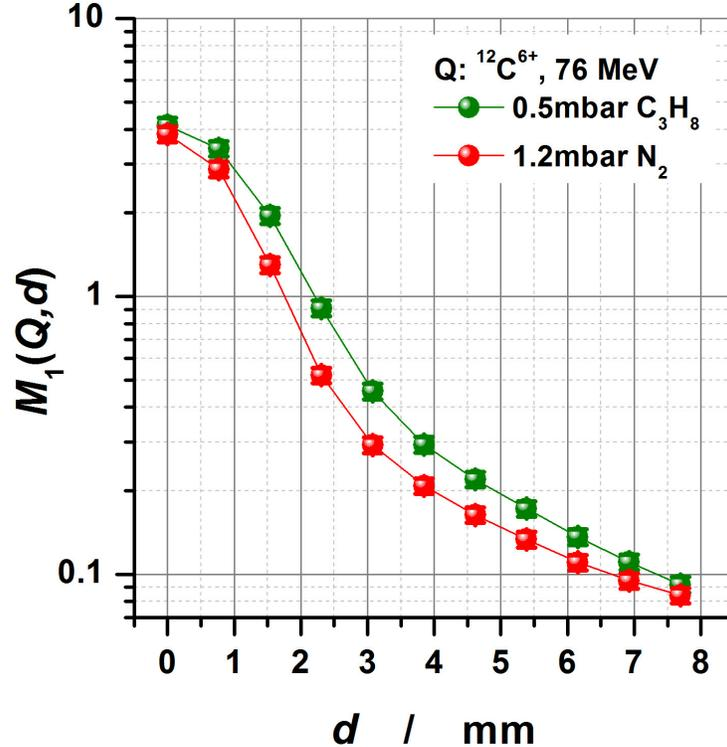
**Figure 2:** Mean ionisation cluster size distributions for 76 MeV  $^{12}\text{C}^{6+}$  ions measured with the PTB Ion Counter in 0.5 mbar  $\text{C}_3\text{H}_8$  and 1.2 mbar  $\text{N}_2$  for different impact parameters  $d$ .
