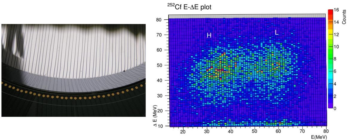
**Figure 3:** Left panel: Connections of four inch thin detector strips with gold PCB bonding pads were performed using 25  $\mu\text{m}$  Al wires. Right panel: Response of 5  $\mu\text{m}$  strip detector to fission fragments from  $^{252}\text{Cf}$  using a collimated single strip detector for the  $E - \Delta E$  telescope.
