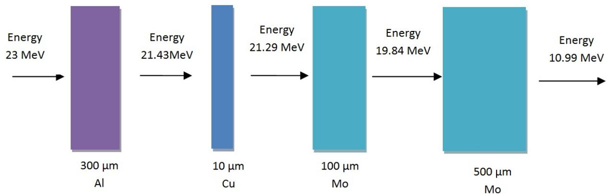
**Figure 1:** Scheme of the irradiated sample with the proton beam energies indicated.
