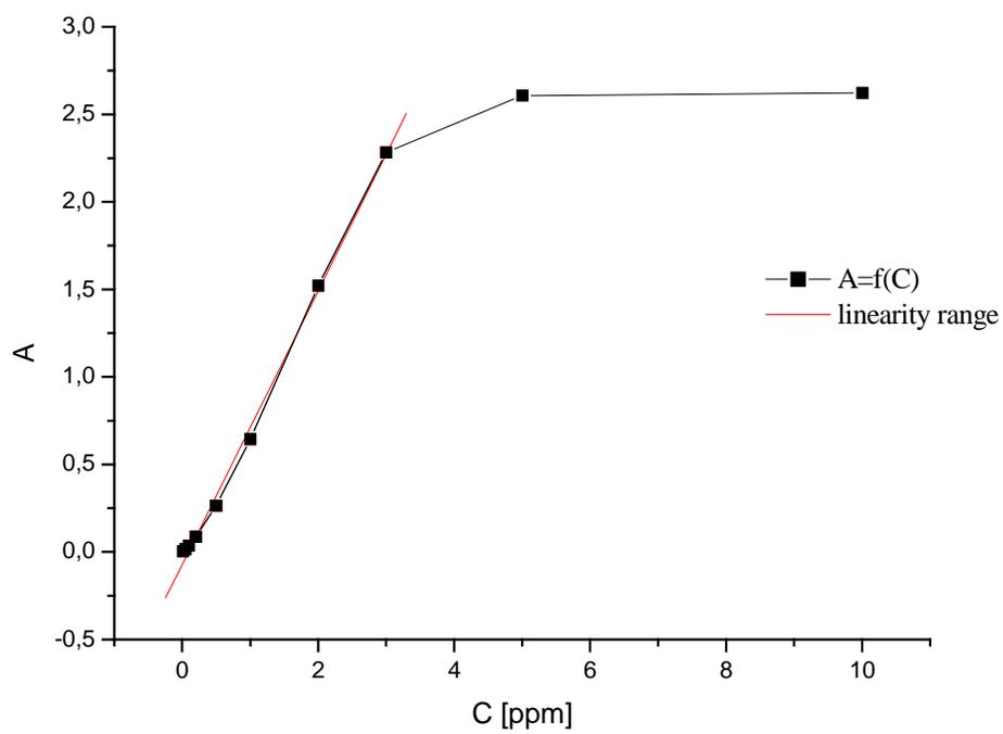
**Figure 1:** Calibration curve for Sc-xylene orange complex.
