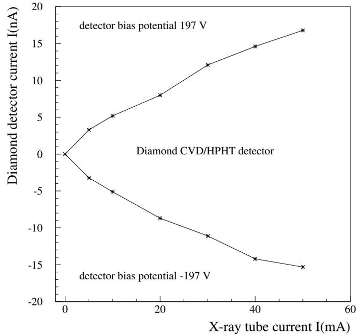
**Figure 3:** Response of diamond CVD/HPHT detector for X-ray fluence generated by X-ray tube current.
