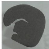
**Figure 2:** Example of a crack passing through the disc about 1 mm thick.
