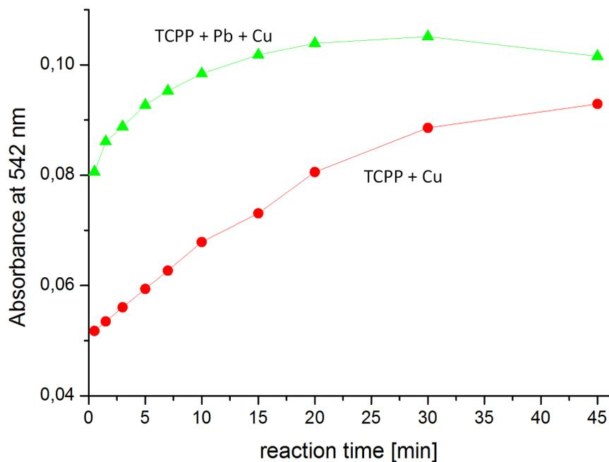
**Figure 2:** The kinetics of CuTCPP complex synthesis using different accelerators.
