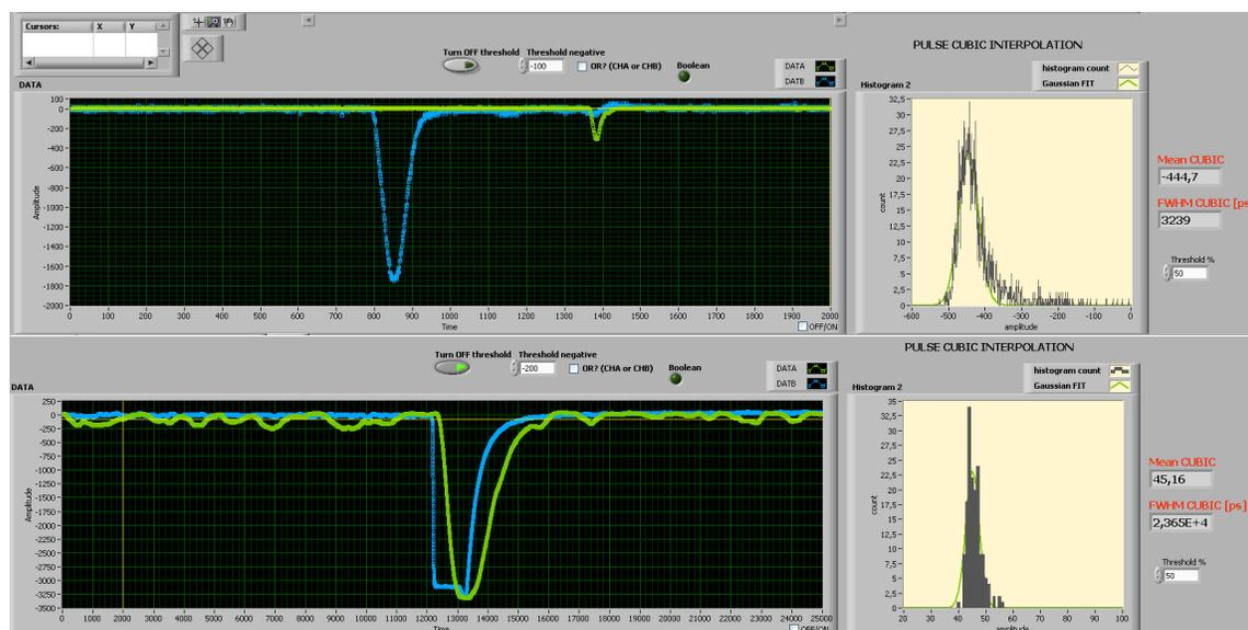
**Figure 2:** The result of the time of flight difference measurements for scCVD (upper) and Si (lower) detectors. Left: signals from the fast amplifiers:  $^{32}\text{S}$  in blue and  $^{107,108}\text{Ag}$  in green. Right: time of flight difference spectrum.
