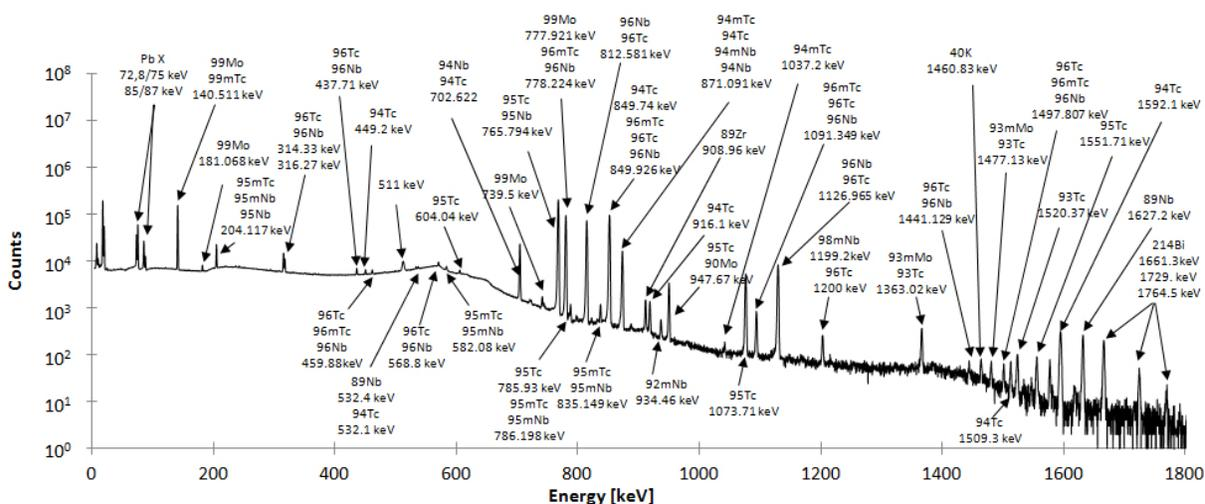
**Figure 2:** Gamma-ray spectrum obtained with a HPGe detector placed at 5.5 cm from the <sup>nat</sup>Mo target of thickness 500 μm irradiated for 13 minutes by protons of 19.84 MeV energy and intensity of 7.16 nA. The measurement was started 26.5 h after EOB. The measurement time was 2.13 h.
