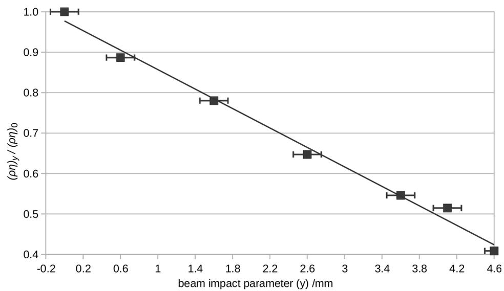
**Figure 2:** Efficiency-density dependence on the beam impact factor for the  $0.32 \mu\text{g}/\text{cm}^2$  nitrogen target in the Jet Counter.
