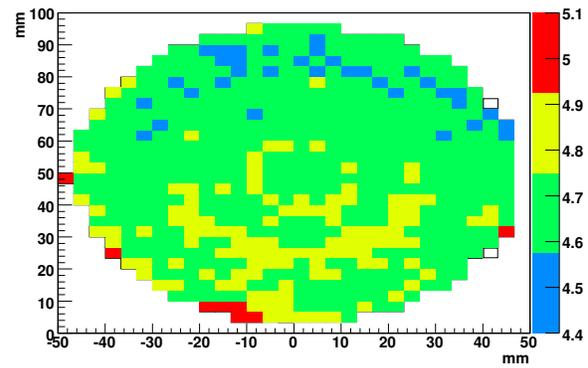
**Figure 2:** Thickness distribution of four inch epitaxial silicon membrane produced by anodic dissolution used for a thin strip detector. Measurements were performed by energy loss of  $\alpha$  particles from an  $^{241}\text{Am}$  source. Colour scale is in microns.
