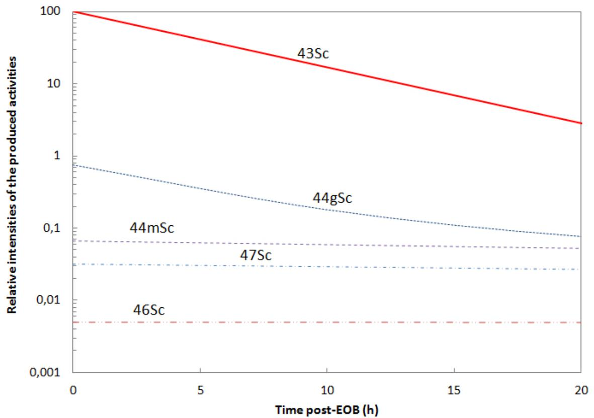
**Figure 1:** Evolution in time of the relative intensities of Sc isotopes produced during a 4 h irradiation of a  $^{nat}\text{CaO}$  target with a 31 MeV  $\alpha$  particle beam.
