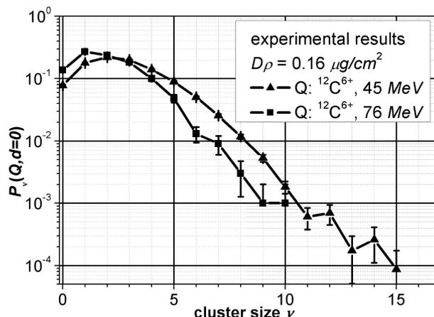
**Figure 2:** Ionization cluster size distributions produced by 45 MeV and 76 MeV carbon ions in  $0.16 \mu\text{g}/\text{cm}^2$  nitrogen nanometric target. NCBJ Jet Counter.
