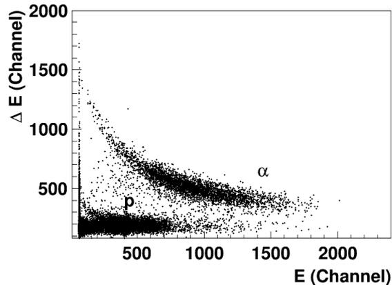
**Figure 2:** Example of the  $\Delta E$ - $E$  particle identification of the  $15^\circ$  telescope.
