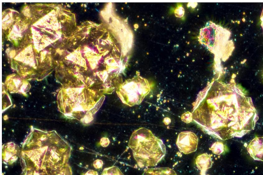
**Figure 1:** Single-crystal diamonds are grown during 8 days on a silicon substrate using 2% concentration of butane in hydrogen at a temperature of about 800°C and a pressure of 70 Th. Randomly oriented diamond crystals of diameter about 0.2 mm are obtained in the hetero-epitaxy process.
