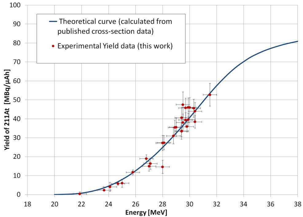
**Figure 2:** The yield of the  $^{211}\text{At}$  production as a function of the  $\text{He}^+$  beam energy.
