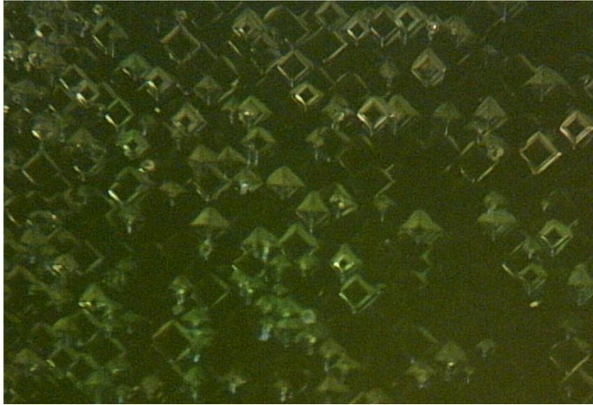
**Figure 2:** [100] oriented diamond single-crystals, grown by MWCVD in the homo-epitaxy process on a [100] diamond Sumimoto substrate. Parallel oriented diamond square pyramids (some of them are without a peak) are visible.
