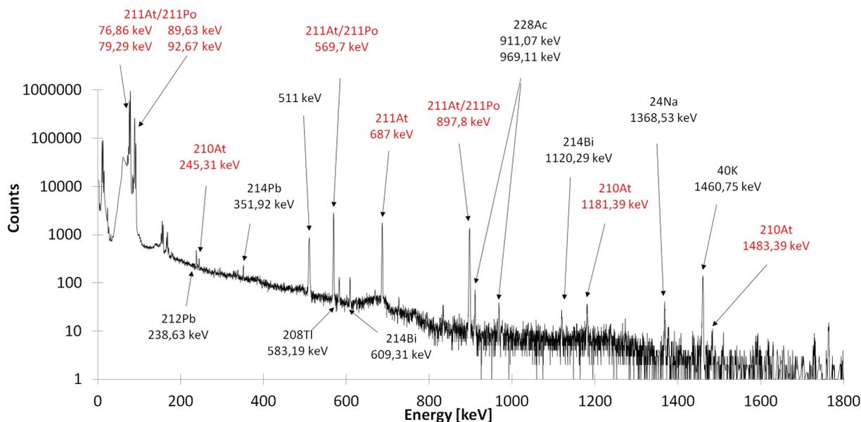
**Figure 1:** Gamma ray spectrum collected with a HPGe detector of 20 % efficiency placed at 86 cm from the bismuth target, irradiated with a 28.5 MeV  $\text{He}^+$  beam of 530 nA intensity during 4.25 h. Measurement time 0.36 h. Beginning of the measurement 1 h after the EOB. The sample activity was 97.5 MBq and the corresponding gamma dose at 30 cm from the sample was  $7 \mu\text{Sv/h}$  at EOB.
