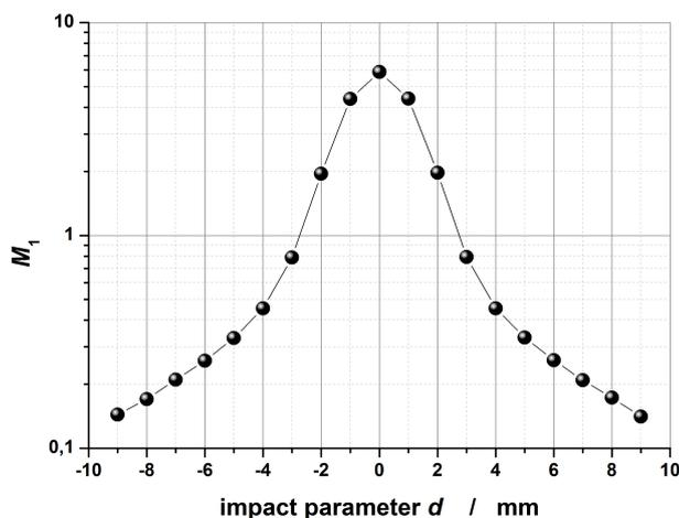
**Figure 3:** Mean ionisation cluster size  $M_1$  for different impact parameters  $d$  measured with the PTB Ion Counter with 45 MeV carbon ions in 1.2 mbar nitrogen.
