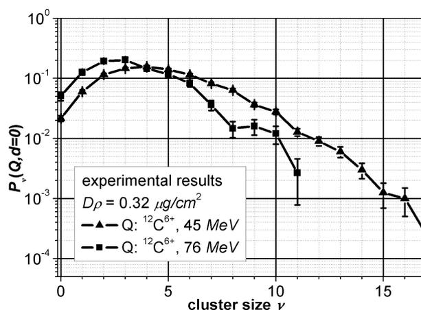
**Figure 1:** Ionization cluster size distributions produced by 45 MeV and 76 MeV carbon ions in 0.16 μg/cm<sup>2</sup> nitrogen nanometric target. NCBJ Jet Counter.
