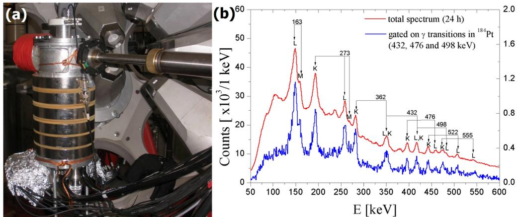
**Figure 1:** The first experiment with the new ICE spectrometer. (a) the spectrometer inside the EAGLE array (b) in-beam electron spectra: inclusive (red line) and exclusive (blue line) gated on  $\gamma$ -transitions in  $^{184}\text{Pt}$ . The transition energies and corresponding electron lines are labelled.
