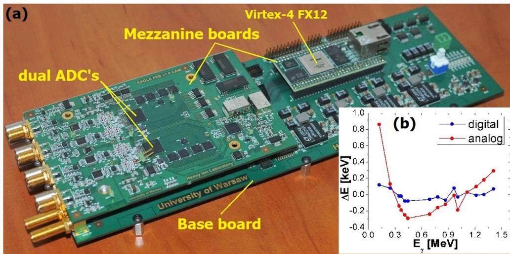
**Figure 2:** (a) The new acquisition module for 4 ACS Ge detectors; the most important components are labelled. (b) The energy difference between actual  $\gamma$ -ray energy and that calculated with linear calibration using  $^{152}\text{Eu}$  source for the presented digital module (blue) and a standard ORTEC analogue amplifier and ADC (red). The lines are drawn only to guide the eye.
