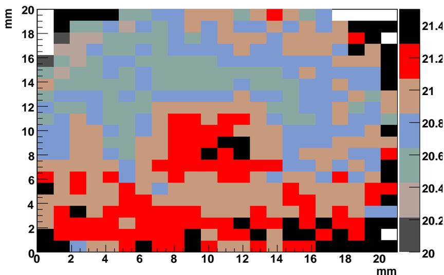
**Figure 1:** Thickness distribution of the epitaxial thin  $\Delta E$  silicon detector. Average value resulting from the map is  $20.9 \mu\text{m}$  and the nonuniformity is within  $1 \mu\text{m}$ . The colour scale is in  $\mu\text{m}$  on the right-hand side of the picture.
