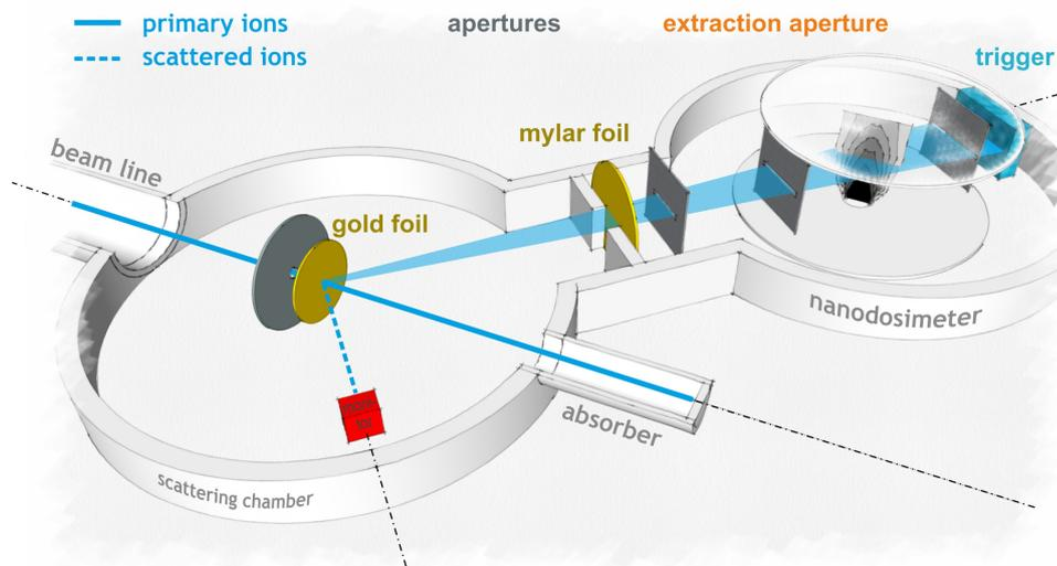
**Figure 1:** Schematic setup of the PTB nanodosimeter for measurements at an ion accelerator.
