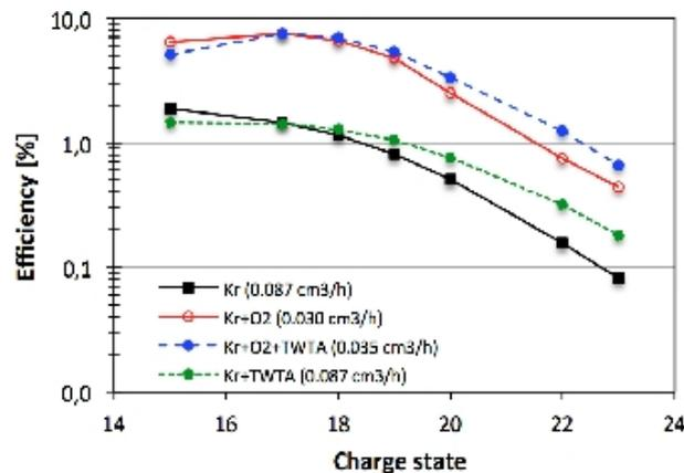
**Figure 7:** Additive effect of 2-frequency plasma heating and gas mixing
