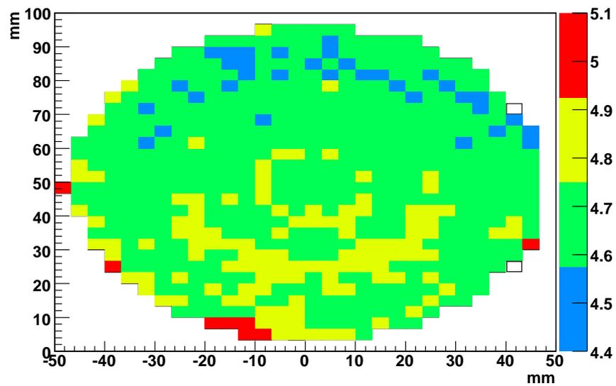
**Figure 3:** Thickness distribution of a 4 in epitaxial silicon layer of thickness below  $5 \mu\text{m}$ . The colour scale is in  $\mu\text{m}$  on right-hand side of the picture.
