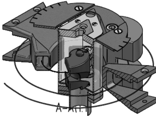
**Figure 6:** The new central part of the cyclotron and spiral inflector.
