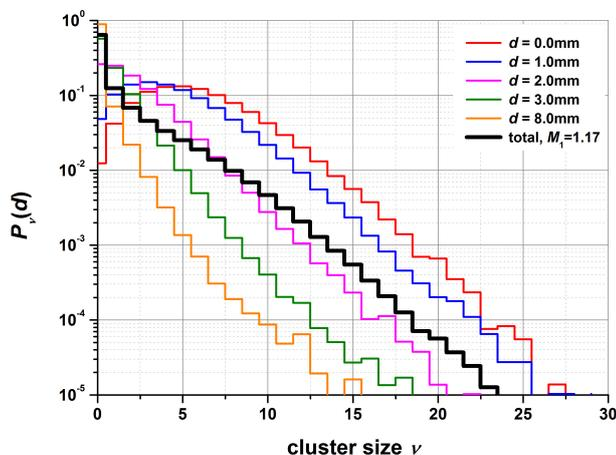
**Figure 2:** Ionisation cluster size distributions  $P_\nu(d)$  at different impact parameters  $d$  and for the total detector size measured with the PTB Ion Counter with 45 MeV carbon ions in 1.2 mbar nitrogen.
