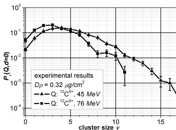
**Figure 3:** The comparison of ICSD spectra measured by the PTB Ion Counter with these measured with the NCBJ Jet Counter. Comparison performed for 45 MeV carbon ions in different targets area densities (see figure).
