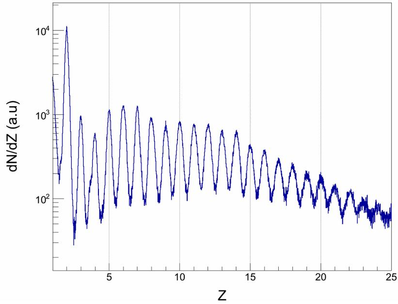
**Figure 2:** Charge distribution of measured ions obtained after linearization of the  $\Delta E - E$  matrix [1].
