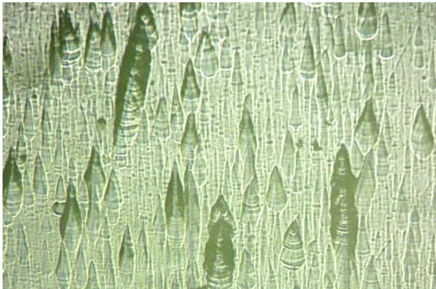
**Figure 3:** Single crystal diamond film of thickness 50  $\mu\text{m}$  grown in 4 days by the MWCVD homo-epitaxy process on a [100] HPHT diamond single crystal Sumimoto substrate.
