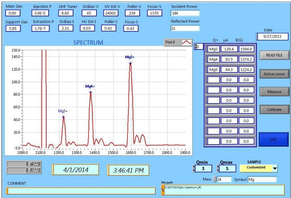
Figure 5: Charge distribution of Mg.
