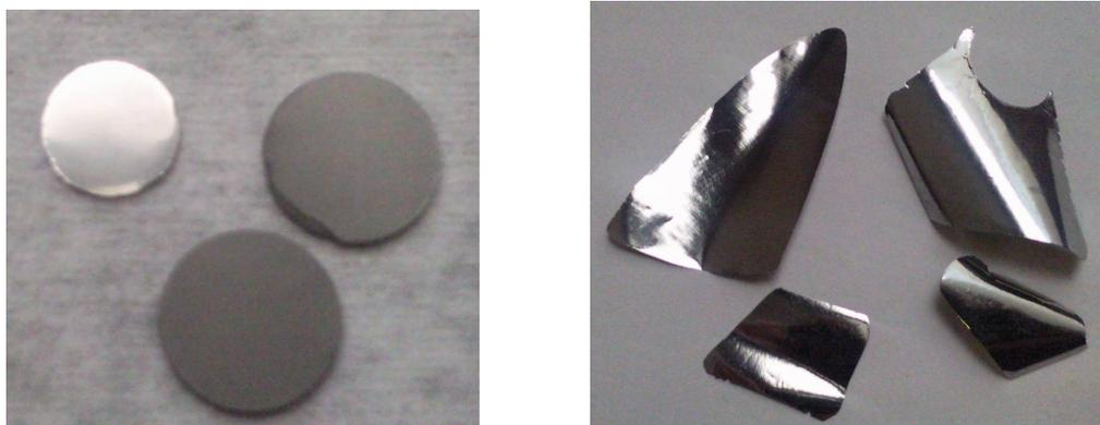
**Figure 1:** Left: Thick Mo-nat pellets of 500 to 2000  $\mu\text{m}$  with density varying from 55 to 85% of the Mo volumetric mass density. Right: Thin Mo-nat foils (10  $\mu\text{m}$ ) prepared by rolling for assembling the “stacked foils” target.
