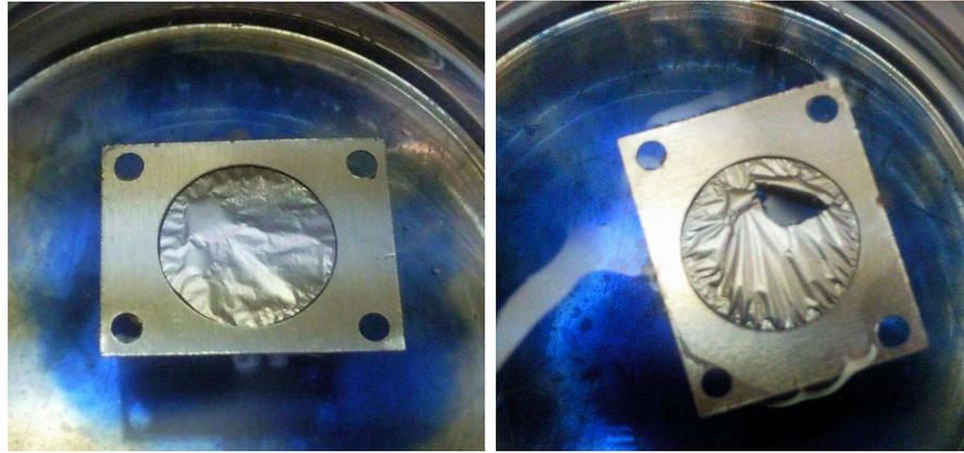
Figure 2: Ni foils prepared on the Cu backing during etching process
