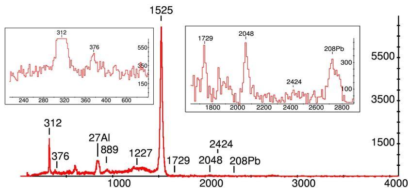
Figure 1: Doppler-corrected  $\gamma$ -ray spectrum observed in the  $^{42}\text{Ca} + ^{208}\text{Pb}$  Coulomb excitation experiment. The insets present 376 keV and 2048 keV  $\gamma$ -ray transitions.
