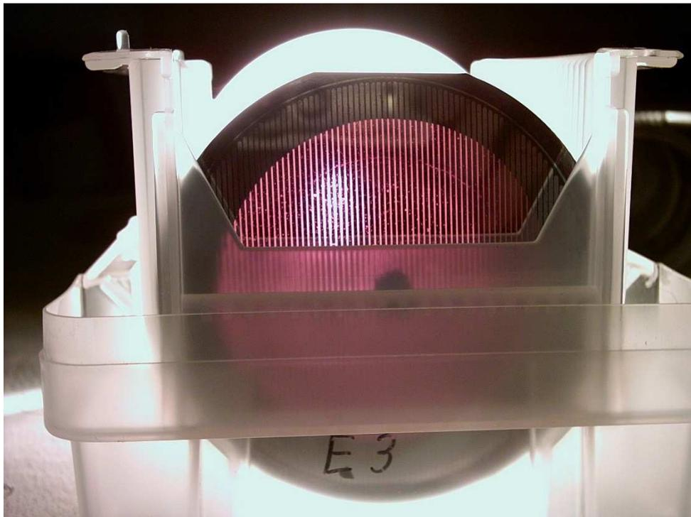
Figure 1: Four inch wafer with 7.3  $\mu\text{m}$  thin silicon membrane supported by a thick 400  $\mu\text{m}$  silicon  $\text{n}^+$  substrate ring. The detector strips are visible in light illuminating the wafer from the back side.
