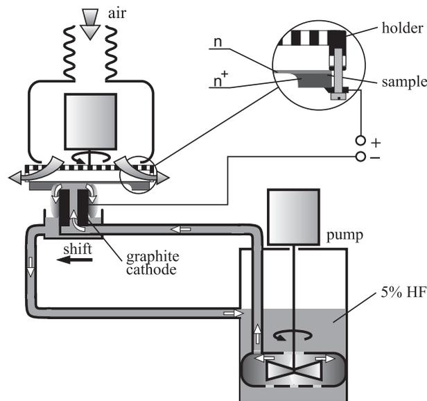
Figure 1: Electrolyte jet technique device used for thinning by anodic dissolution the large-area  $n^+$ - $n$  oxidated silicon epitaxial wafers. After attaching an opposite voltage, the reverse current of the silicon/liquid 5% HF junction was observed.
