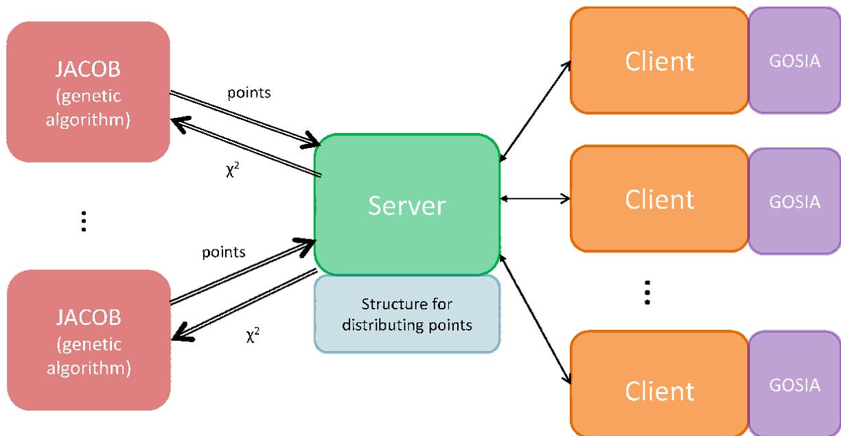
Figure 1: The distributed architecture of the system.
