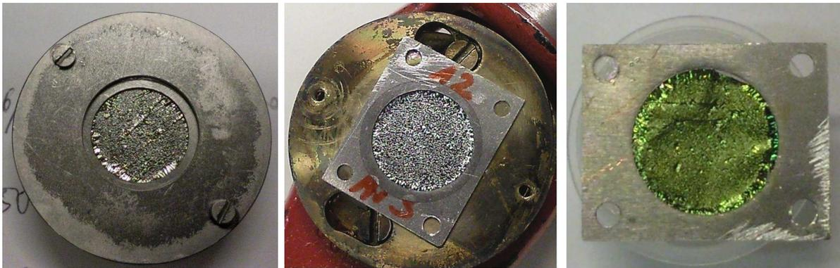
Figure 3: Left: the Ni target in the holder of the sputtering device (from the Ni side). Centre: the circle of the nickel (darker grey ring) on the frame guarantees the nickel contact with the frame to facilitate the heat transfer from the target material. Right: view of the target from the PIF side.
