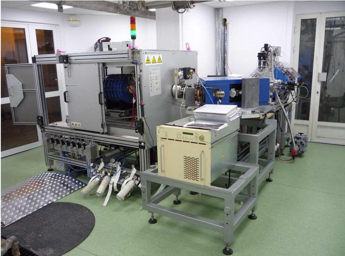
Figure 2: New ECR ion source with the the horizontal part of injection line
