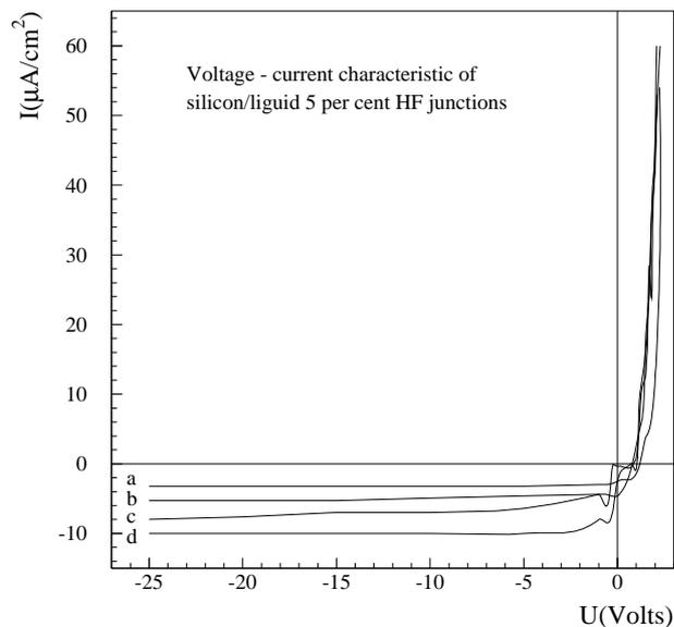
Figure 2: Voltage-current characteristics of silicon/liquid 5% HF junctions. (a) High resistivity silicon. Float zone. Tewa. (b) High resistivity silicon. Float zone. Topsil. Open circuit voltage 0.83 V. (c) High resistivity silicon epitaxial  $n^+$ -n. ITME. Open circuit voltage 0.63 V. (d) High resistivity silicon epitaxial  $n^+$ -n. ITME. Open circuit voltage 0.68 V. All voltages were measured with light illumination of junctions.
