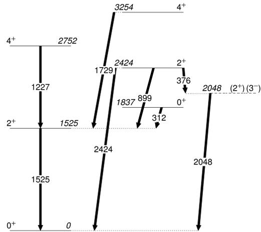
Figure 2: The level scheme of  $^{42}\text{Ca}$  observed in the present experiment with the tentatively assigned  $3^-$  or  $2^+$  state at the energy of 2048 keV.
