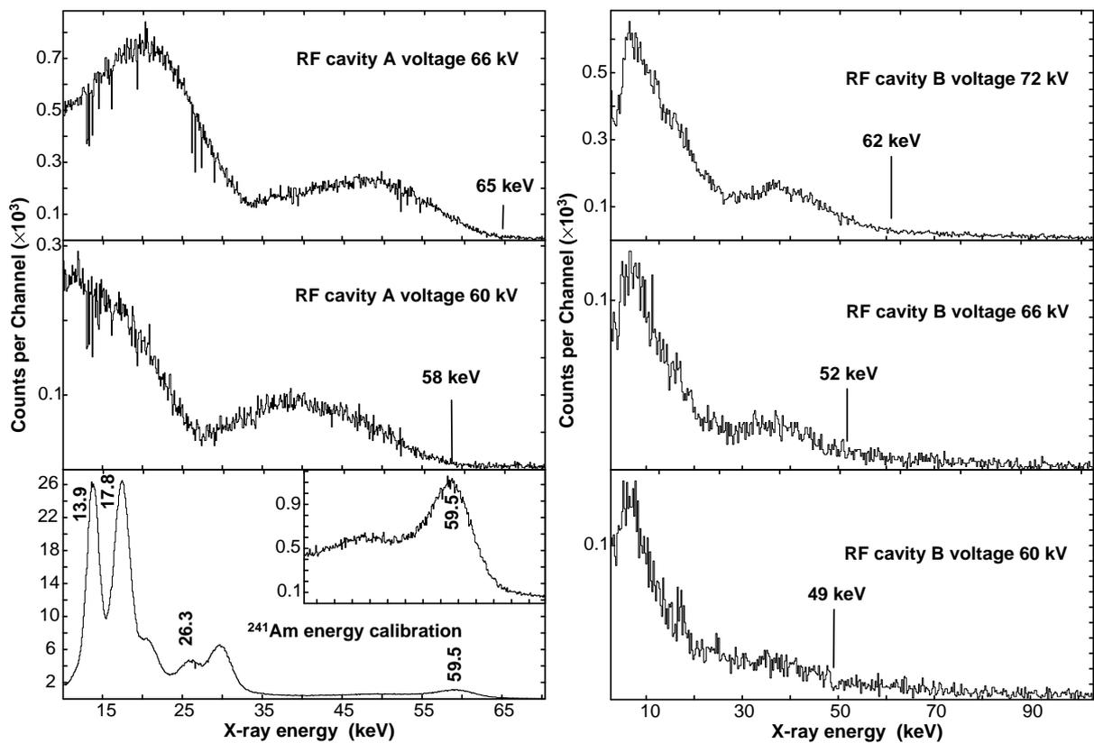
Figure 1: X-ray spectra for the two RF-cavities for three different voltmeter voltages (60, 66 and 72 kV) and the 15 MHz RF frequency. The  $^{241}\text{Am}$  X-ray calibration spectrum is also shown. The measured voltages are marked in the plots.
