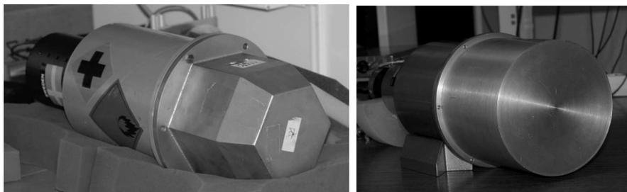
Figure 1: Neutron detectors used in the test measurements – the NORDBALL H10 detector evaluated in Uppsala (left) and a cylindrical detector tested in Warsaw (right).
