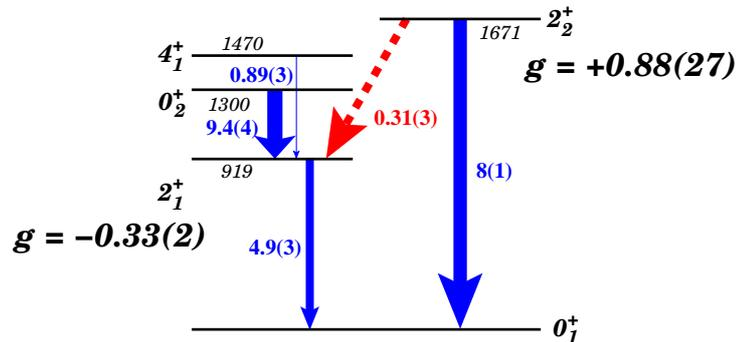
Figure 1: Available experimental information of  $^{94}\text{Zr}$  previous to our experiment. The reduced transition probabilities (E2: solid line, M1: dashed) are given next to the arrows indicating the transitions.
