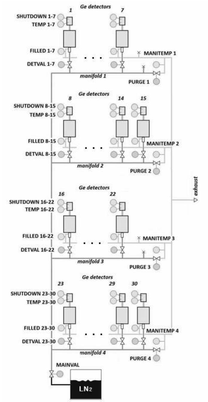
Figure 1: Scheme of the EAGLE LN<sub>2</sub> filling installation.
