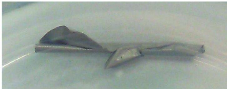
Figure 1: Ni foil made by sputtering on the Cu backing after etching the backing.
