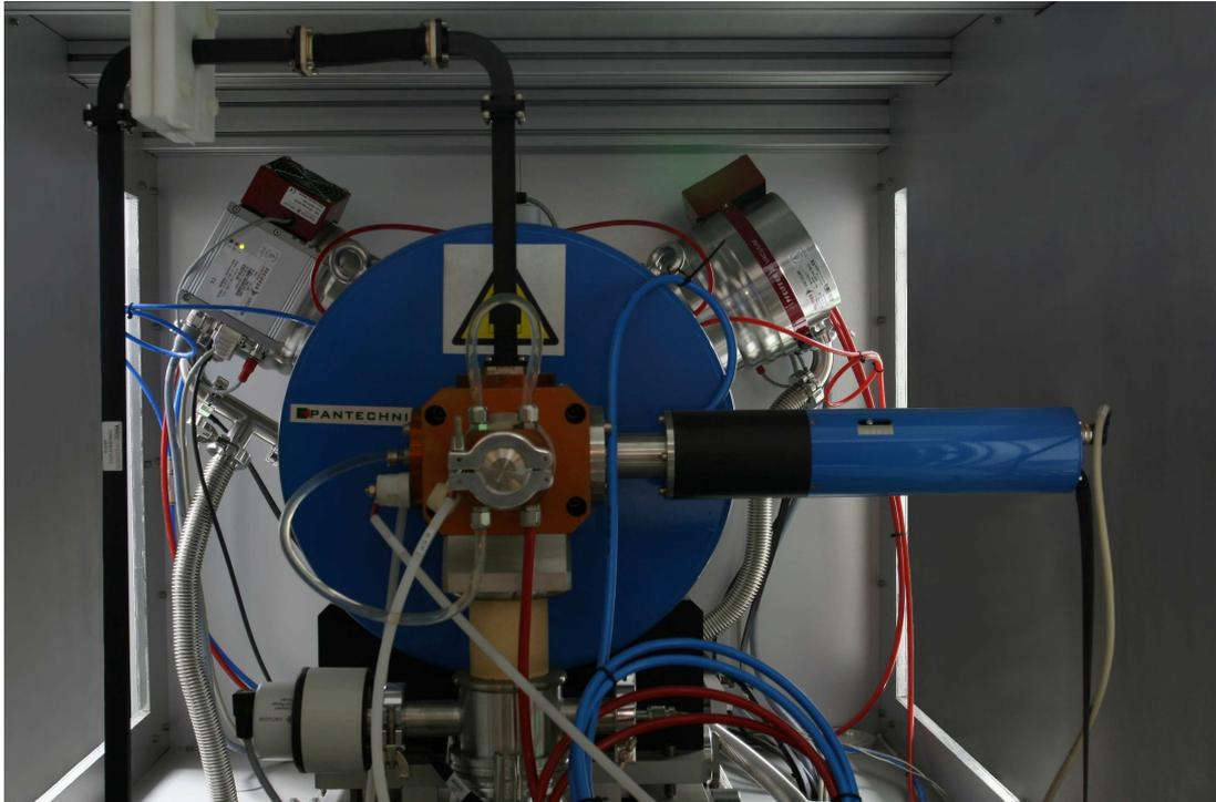
Figure 1: New ECR ion source with its shielding
