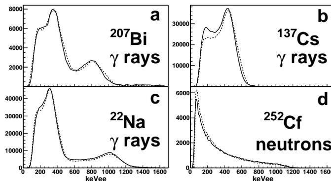
Figure 2: Experimental (solid line) and simulated (dotted) spectra obtained with the NORDBALL detector for  $\gamma$ -ray sources  $^{22}\text{Na}$  (a),  $^{207}\text{Bi}$  (b) and  $^{137}\text{Cs}$  (c); as well with the cylindrical detector for neutrons emitted by the  $^{252}\text{Cf}$  source (d). Neutrons were distinguished from  $\gamma$  rays using the charge-comparison method.
