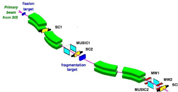
Fig.1 Experimental set-up including Fragment Separator (FRS) magnets
