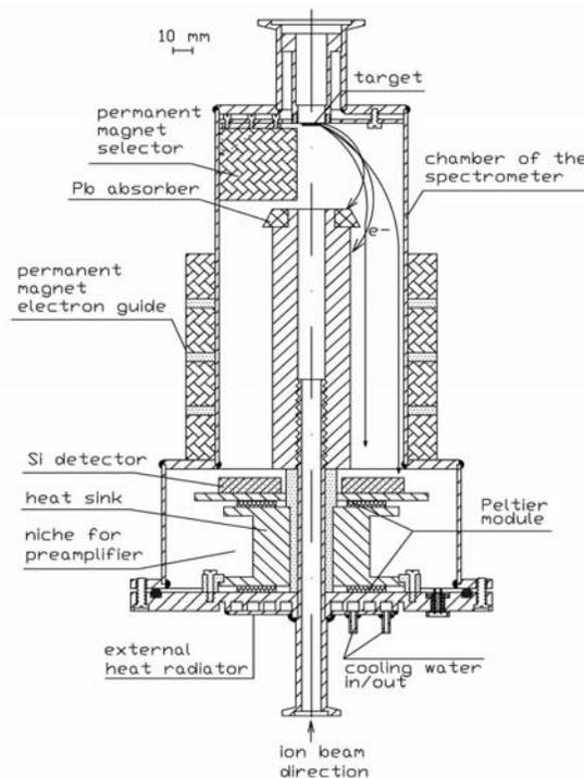
Figure 1. Cross-section of the internal electron spectrometer.
