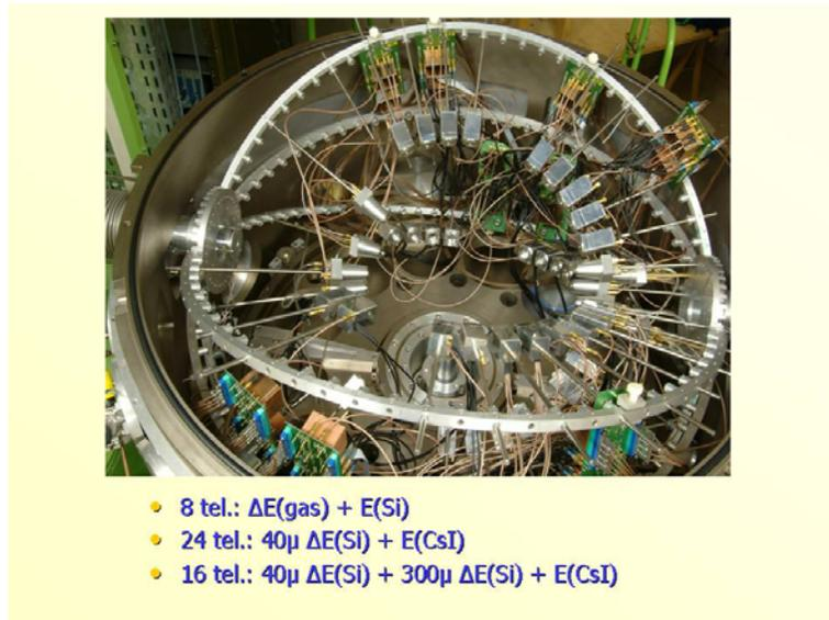
Fig. 2. Telescopes mounted inside the ICARE reaction chamber
