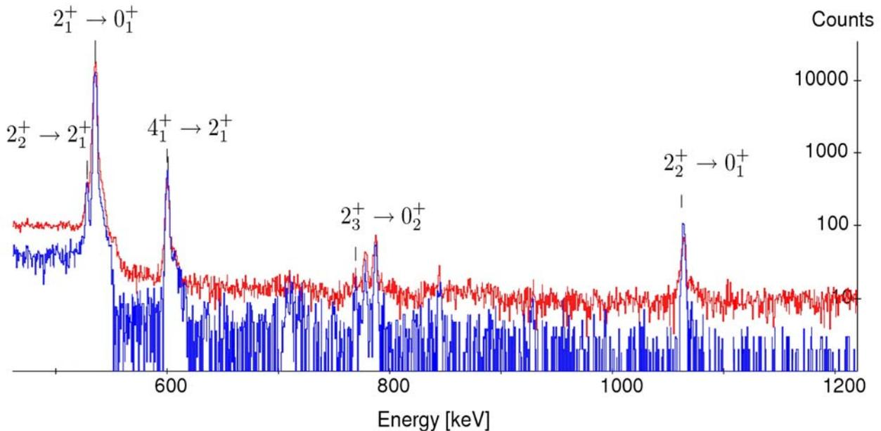
**Figure 1.** Red: Gamma-ray spectrum in coincidence with  $^{20}\text{Ne}$  projectiles scattered on a  $^{100}\text{Mo}$  target collected by a single HPGe detector in coincidence with the CUDAC particle detection set-up.
