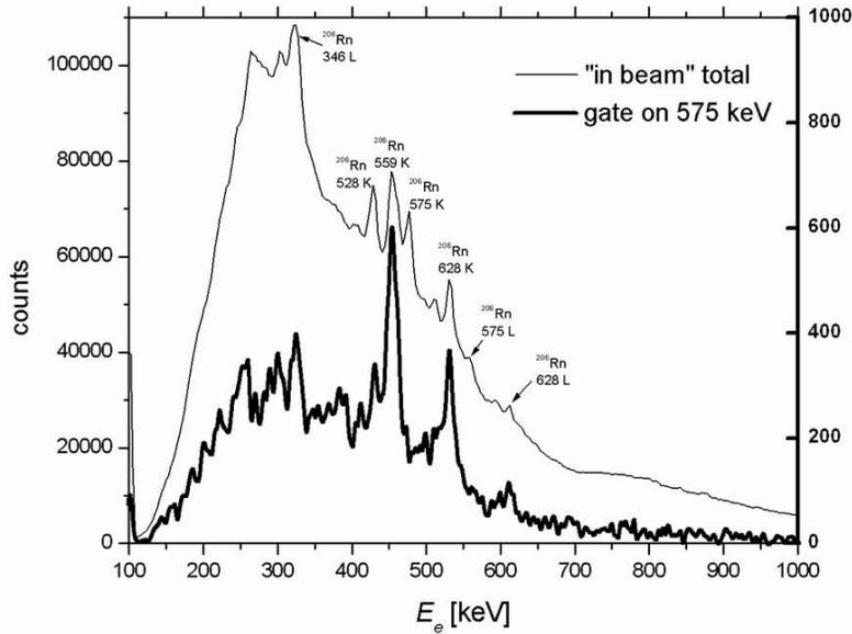
Figure 3. Spectrum of internal conversion electrons measured “in beam” (thin line), and spectrum of internal conversion electrons in coincidence with gamma ray at the energy 575 keV from the  $^{206}\text{Rn}$  (thick line).
