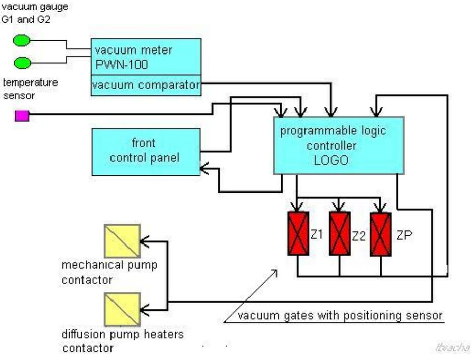
Figure 1 The bloc diagram of the universal control unit “Ania”
