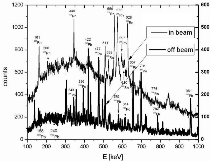
Figure 2. The gamma-ray spectra measured during the experiments. The peaks from the  $^{206}\text{Rn}$  and daughter nuclei are labelled.
