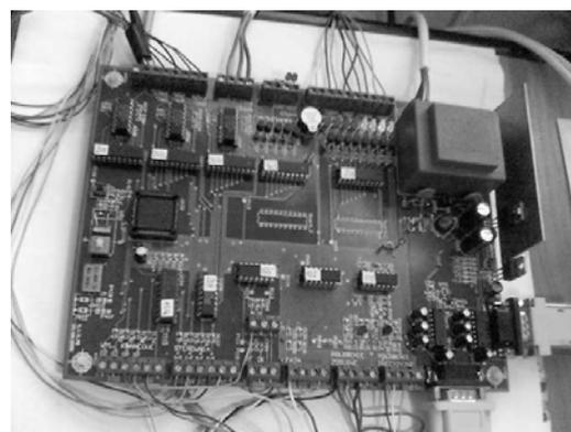
Fig.2 New microprocessor controller
