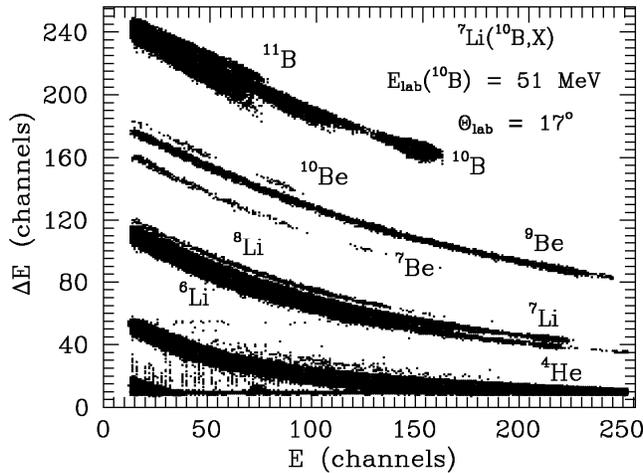
Fig. 1. Typical  $\Delta E(E)$ -spectrum from the  ${}^7\text{Li}({}^{10}\text{B}, X)$  reactions at energy  $E_{\text{lab}}({}^{10}\text{B}) = 51 \text{ MeV}$  for the angle  $\theta_{\text{lab}} = 17^\circ$ .
