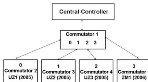
Fig.1 Structure of ZM1 controller communication network
