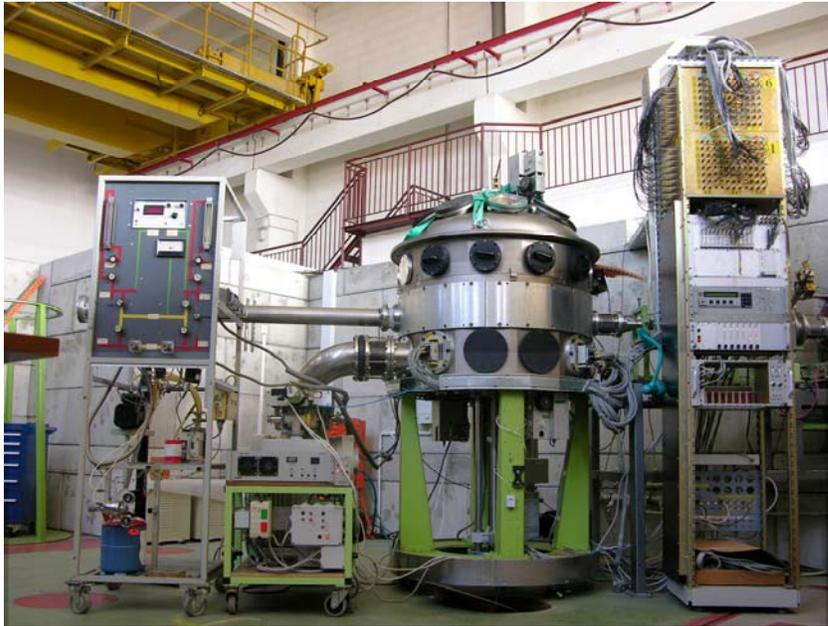
Fig.1 External view of the ICARE reaction chamber with vacuum and gas system.
