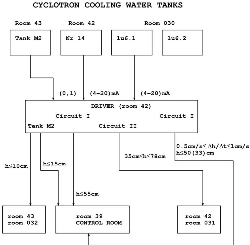
**Fig.1.** Block scheme of the cooling circuit.
