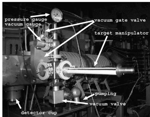
**Fig. 1.** Beam diagnostics system attached to the diagnostics box. Two main components attached to a diagnostic box can be seen: detector cup (lower left side) and target airlock vacuum system (center).
